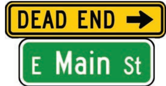
Figure 18: Placement of W14-1a sign with street name (D3-1) sign
