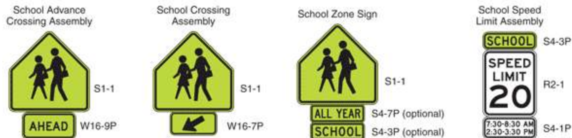
Figure 7B-1. School Area Signs
