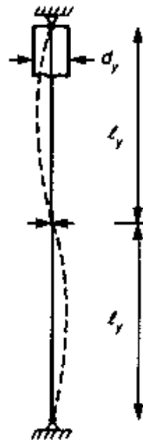
Buckling mode about the y-y axis (\ell_o/d)_y
