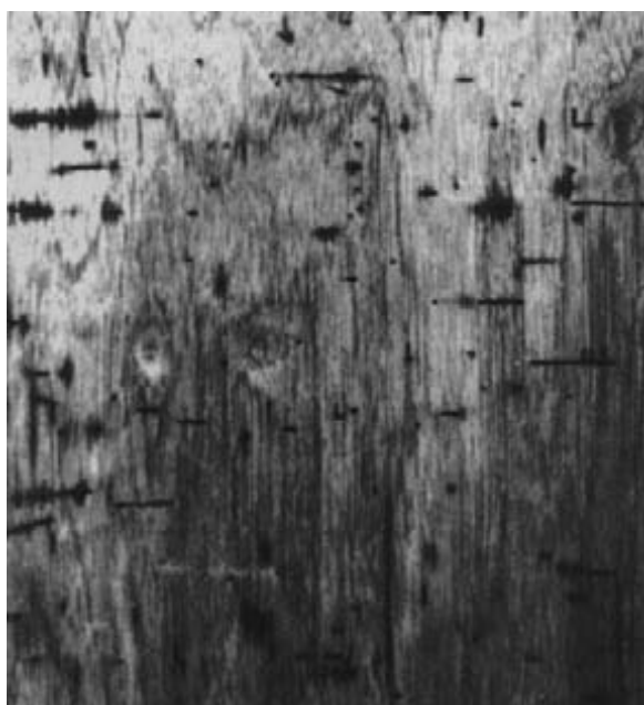
Figure 13-11. - Damage by Ambrosia beetles in green wood. The galleries are free of residue and the surrounding wood is darkly stained.
