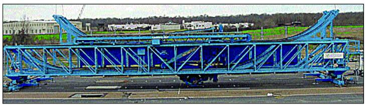
Accelerated Loading Device at Pavement Research Facility
