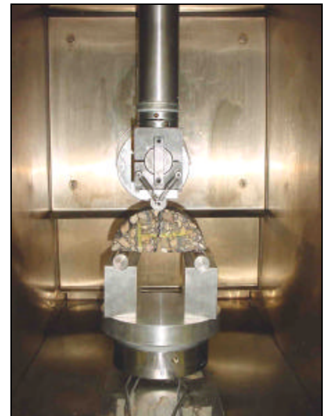
Bend testing of semi-circular specimen of compacted asphalt mixture
