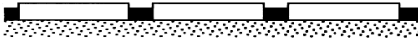
Fig.2 Illustrating the effect of aggregate particle shape on materials quantities. Both aggregates are 0.5 inch as measured by sieve analysis. One is cubicle, the other is flat and elongated. Voids filled is 70% for both aggregates.
