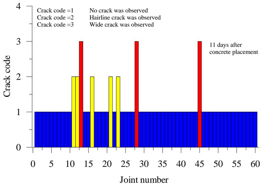
(b) Test section S2 with early entry dry cut narrow joints
