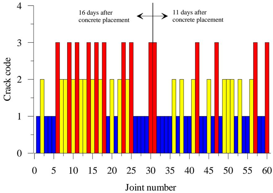
(a) Control section (S1) with wet cut standard joints
