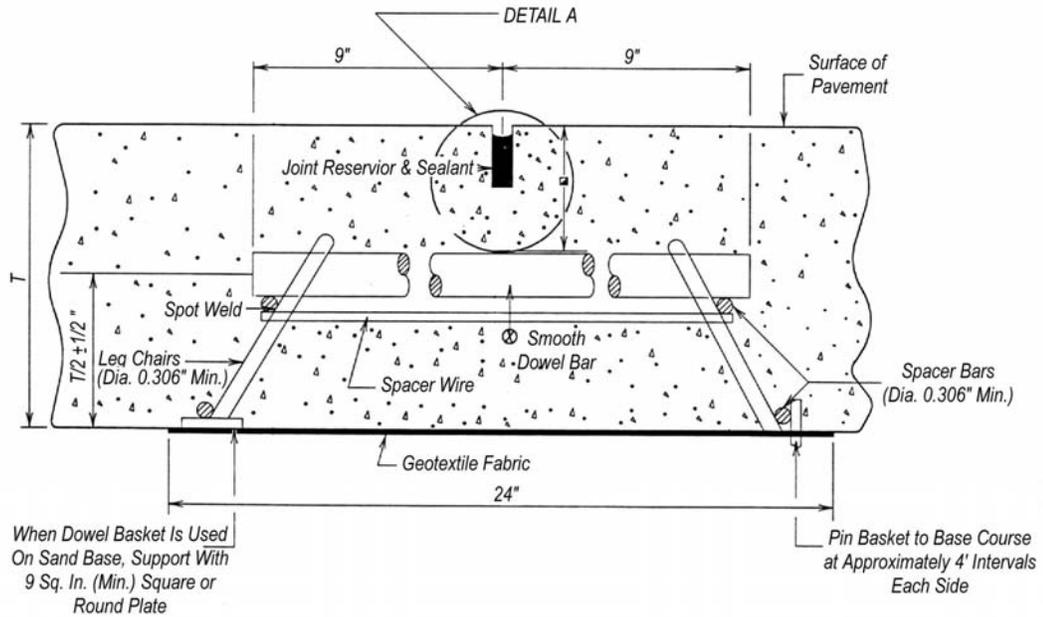
(a) The general configuration of transverse contraction joints
