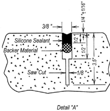
(b) The most common type of transverse contraction joints
