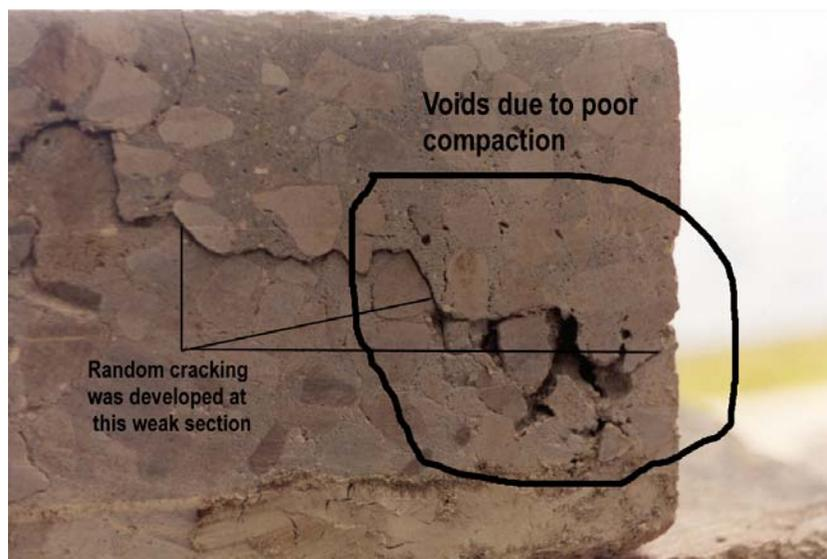
(b) Poor construction practice resulted in development of random cracking within the concrete pavement slab
