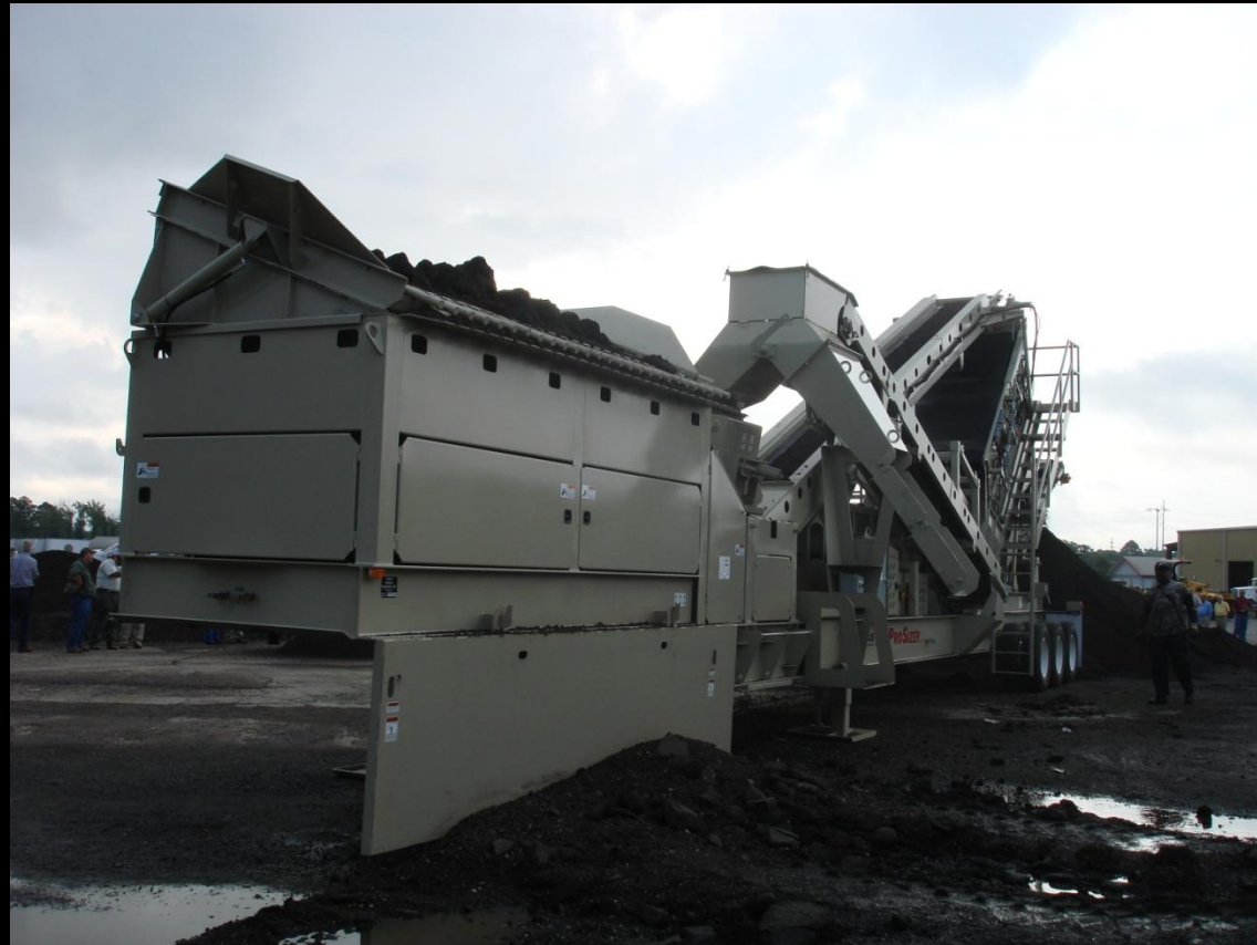
RAP Sizing Plant
