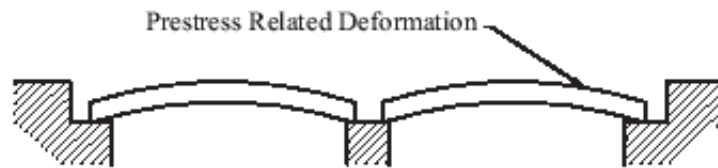
Simply supported girders: stage one of construction.
