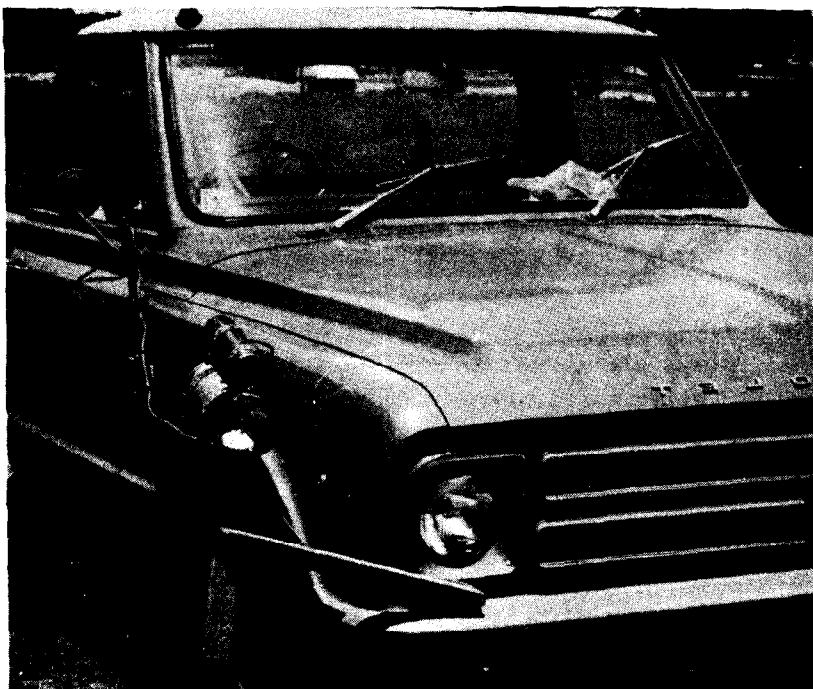
Vehicle Mounted Reflectivity Testing Device FIGURE 13a
