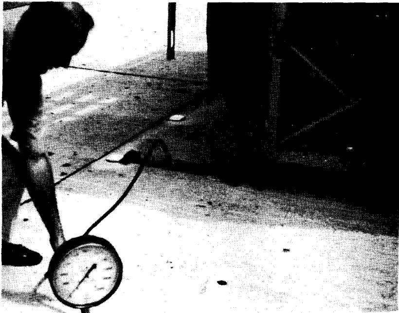
Rig Used for Field Testing of Epoxy Bonding FIGURE 27
