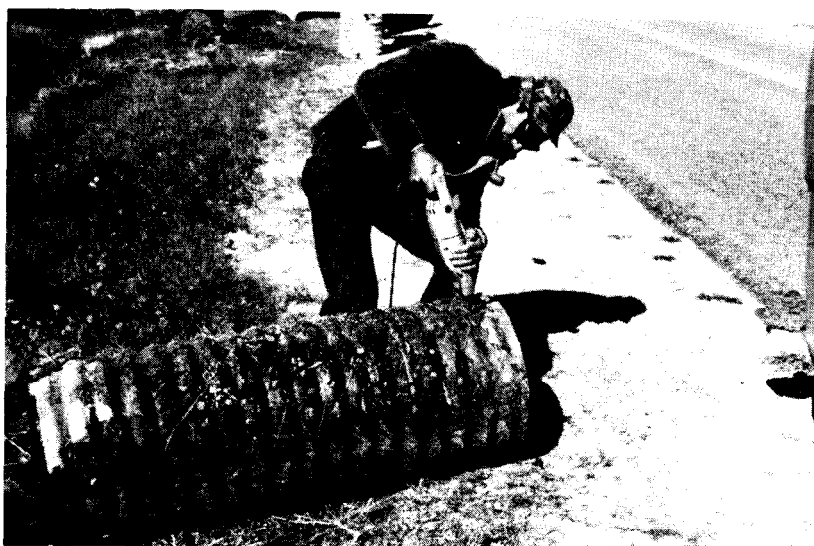
Cutting Sample for Laboratory Testing FIGURE 6
