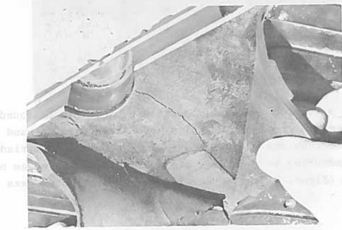
Internal Fracturing Propagating From Cutouts
