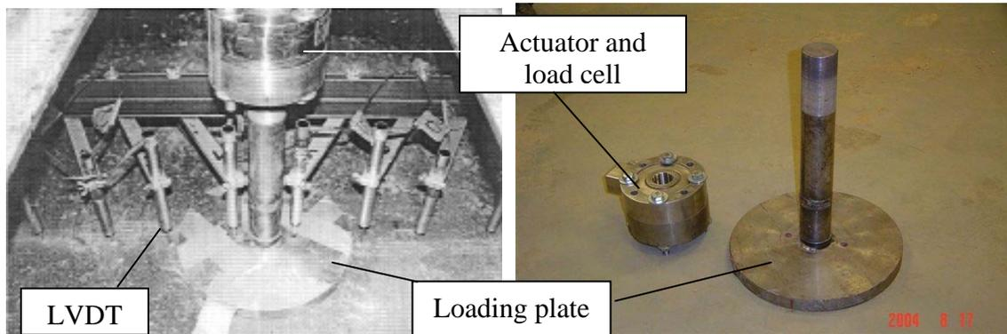
**b) Loading and rutting measurement**
