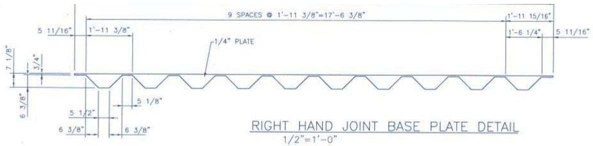
**Figure 4: Tongue and groove "finger" joint bottom section (source Tri-Dyne)**
