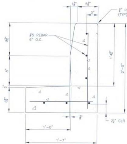
**Figure 6: Curb detail (source Tri-Dyne)**
