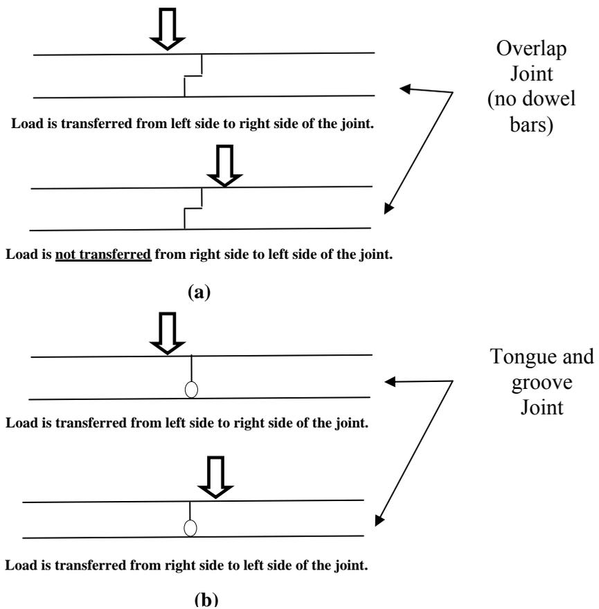
**Figure 7: Load transfer detail for joints**
