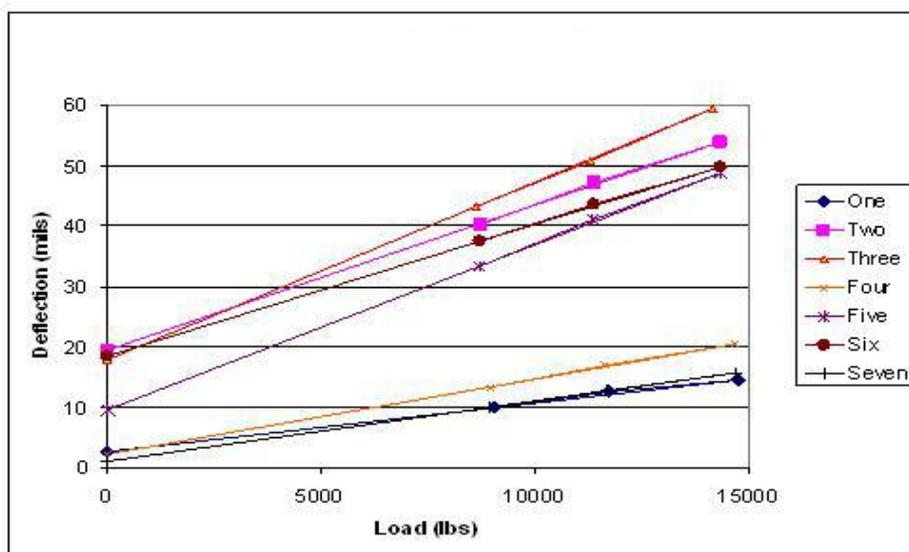
**Figure 9: Y intercept diagram for void**
