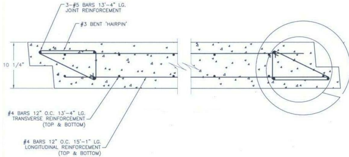
**Figure 3: Overlap joint detail (source Tri-dyne)**
