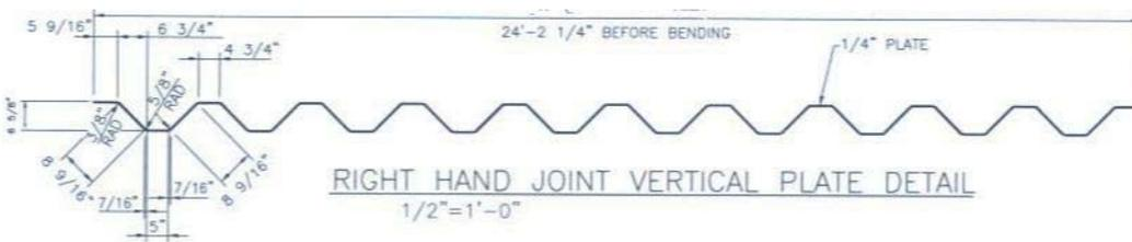
**Figure 5: Tongue and groove joint top section (source Tri-Dyne)**
