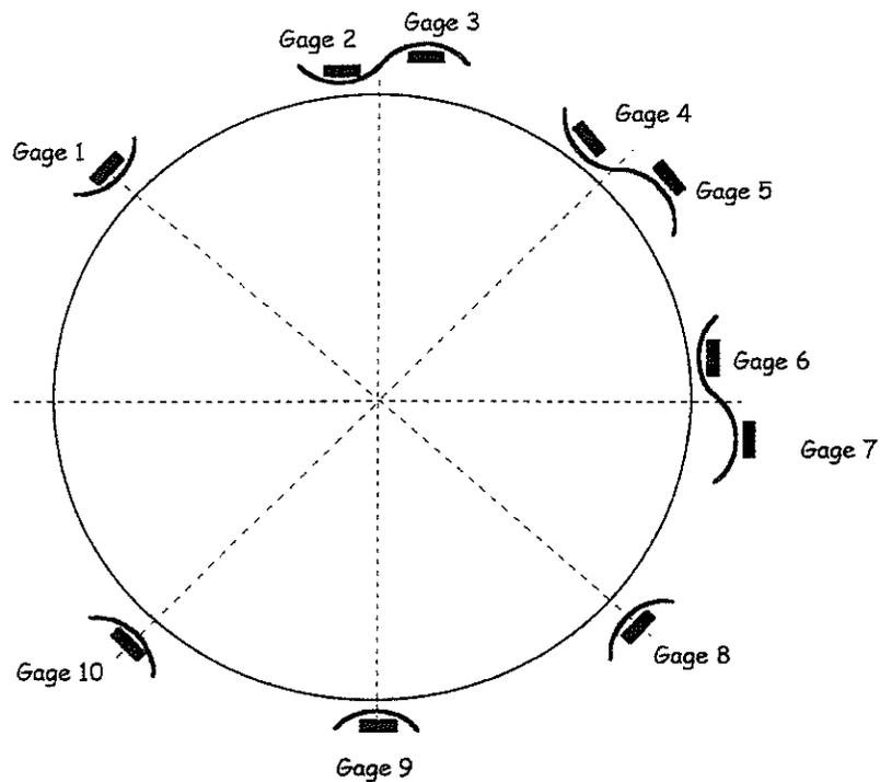
Figure 31. Schematic of the strain gages locations in the lab
