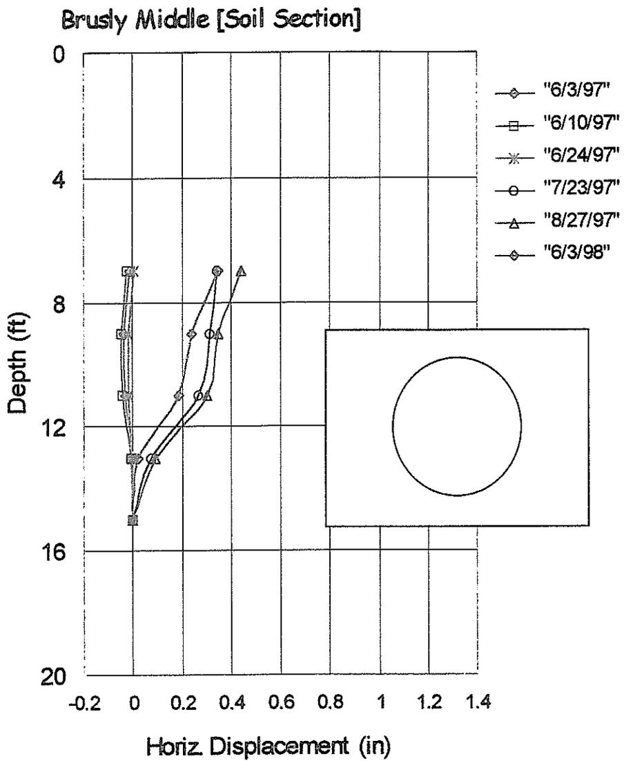
Figure 20. Horizontal soil displacement near the pipe in the soil section
