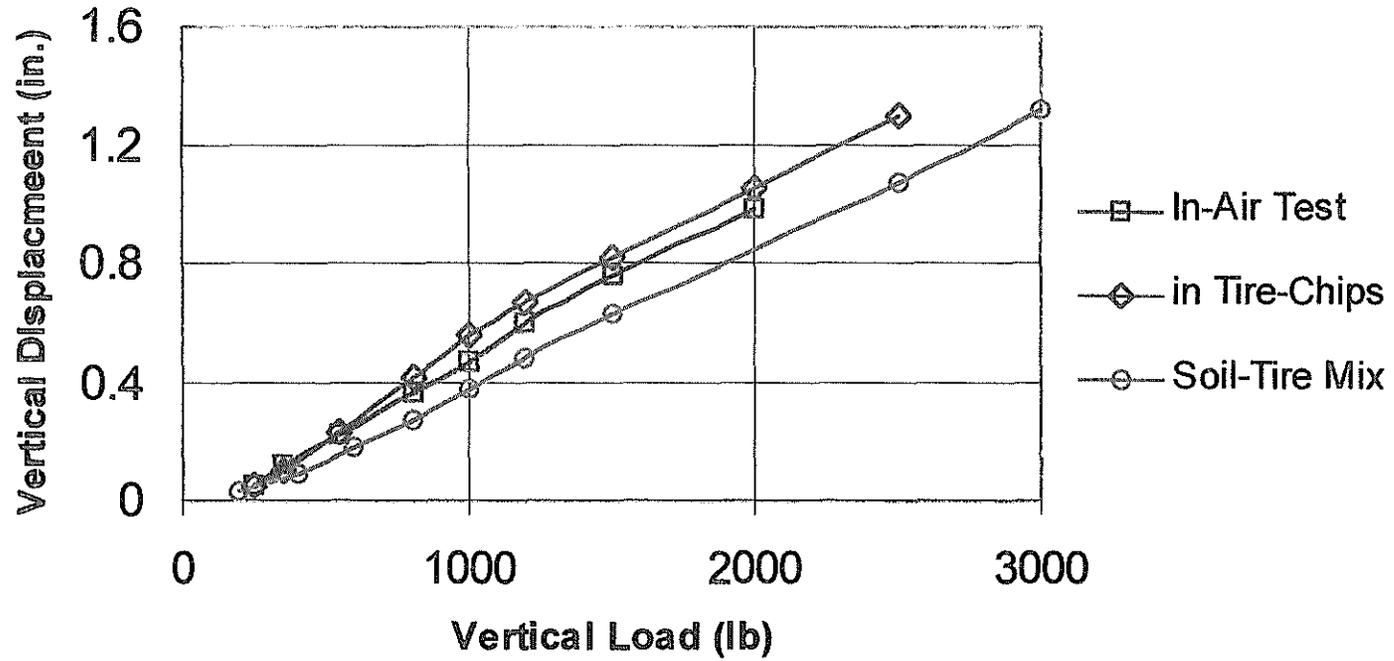
Figure 41. Measurements of vertical pipe displacement by the LVDT
