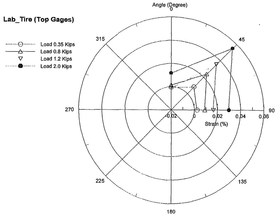
Figure 37. Strain measurements of top gages in tire fill
