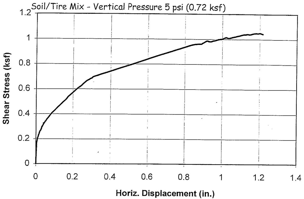
Figure A-5 Direct shear test on soil-tire mix
