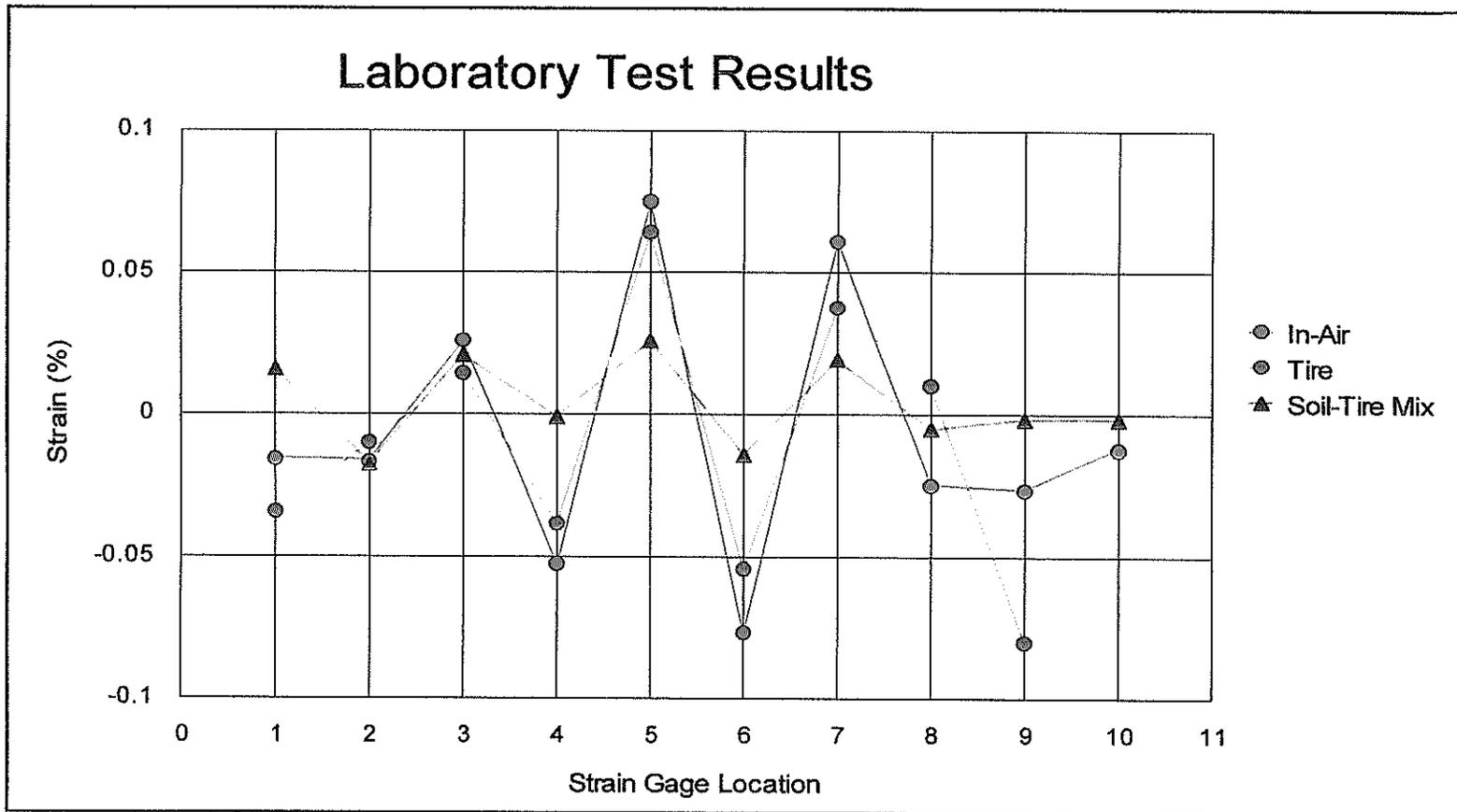
Figure 40. Comparison of strain gages measurements in the laboratory
