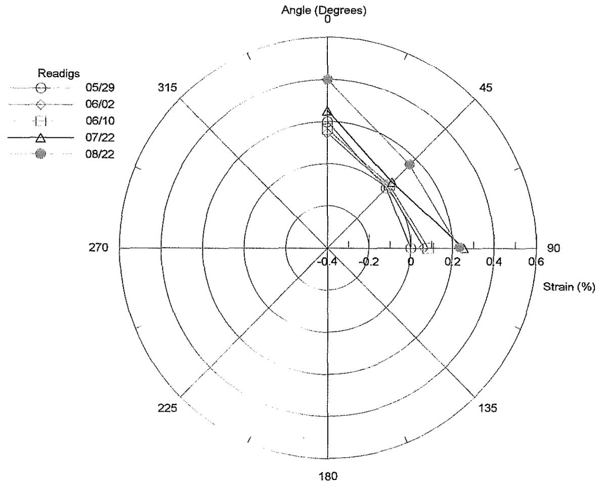
Figure 24. Strain measurements of top gages in the soil section
