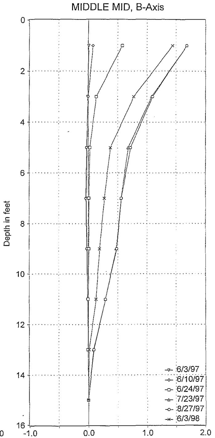
Figure B-3 Vertical Inclinometer readings in soil section
