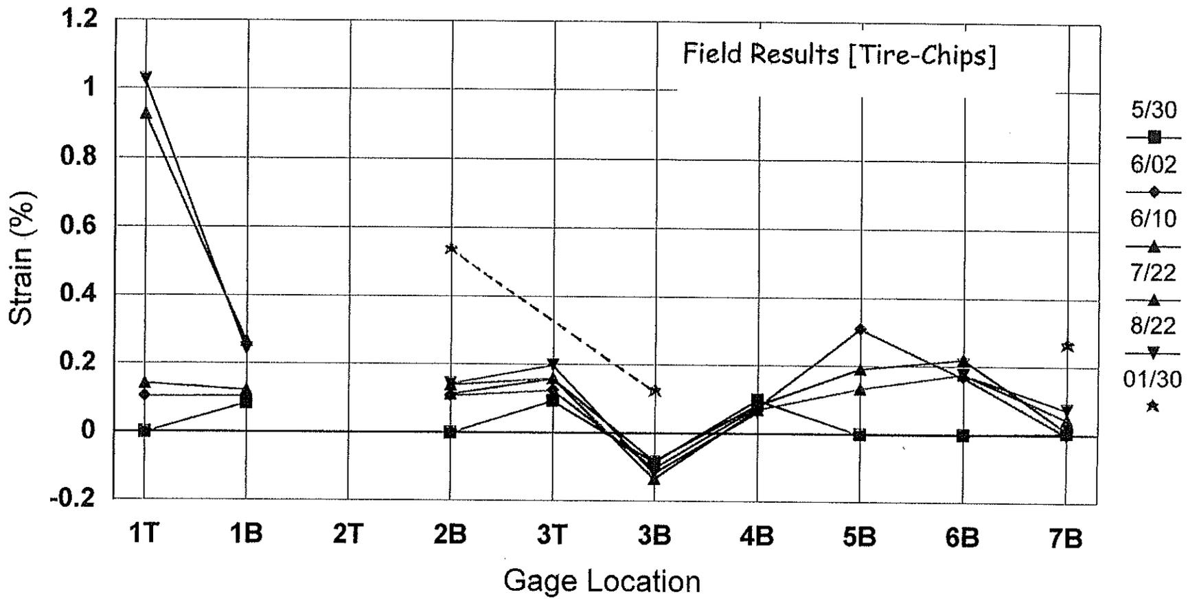
Figure B-4 Strain gage readings in tire section [see figure 14 for gage locations]
