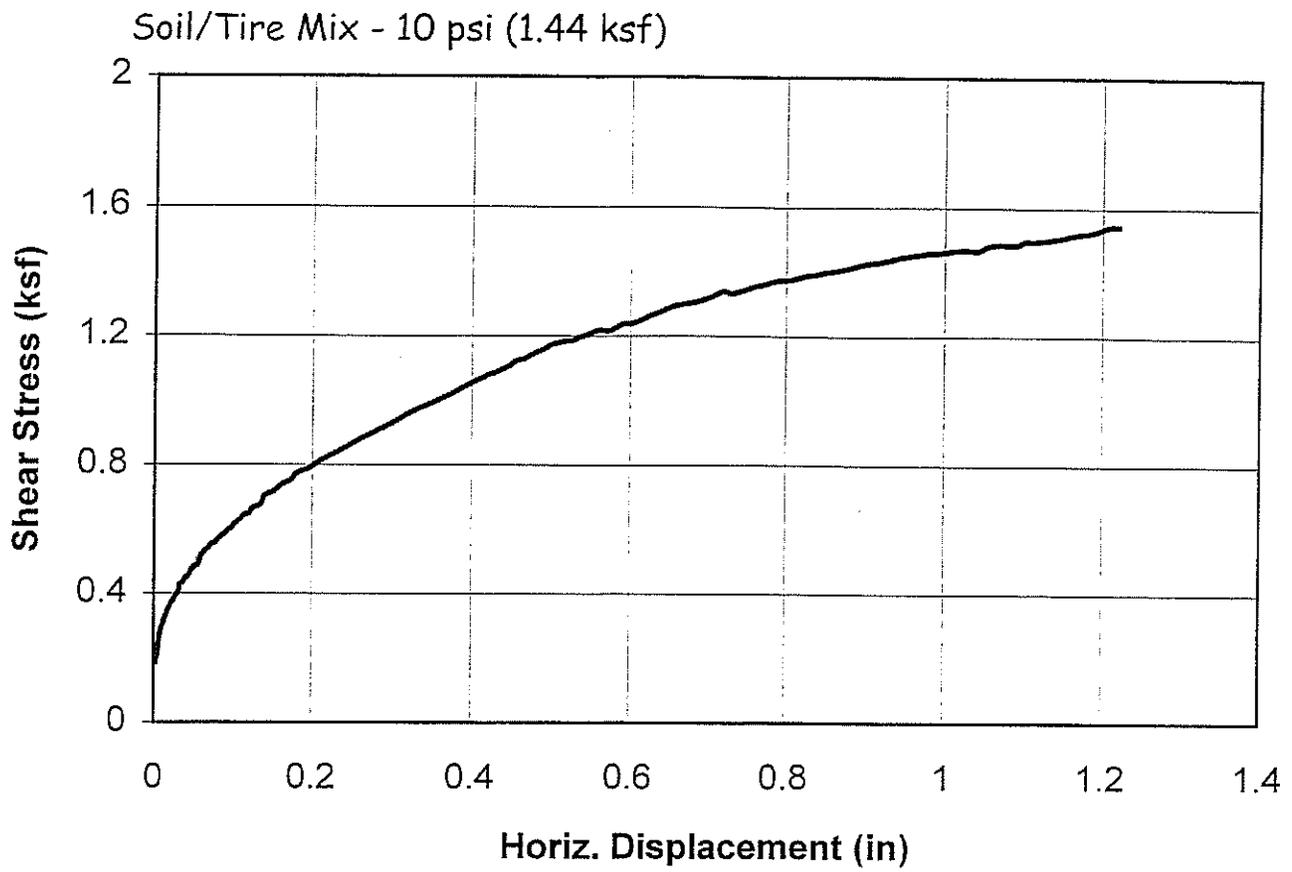
Figure A-6 Direct shear test on soil-tire mix
