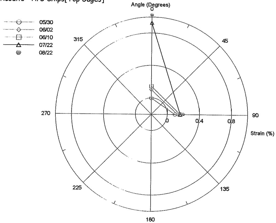
Figure 28. Strain measurements of top gages in the tire section
