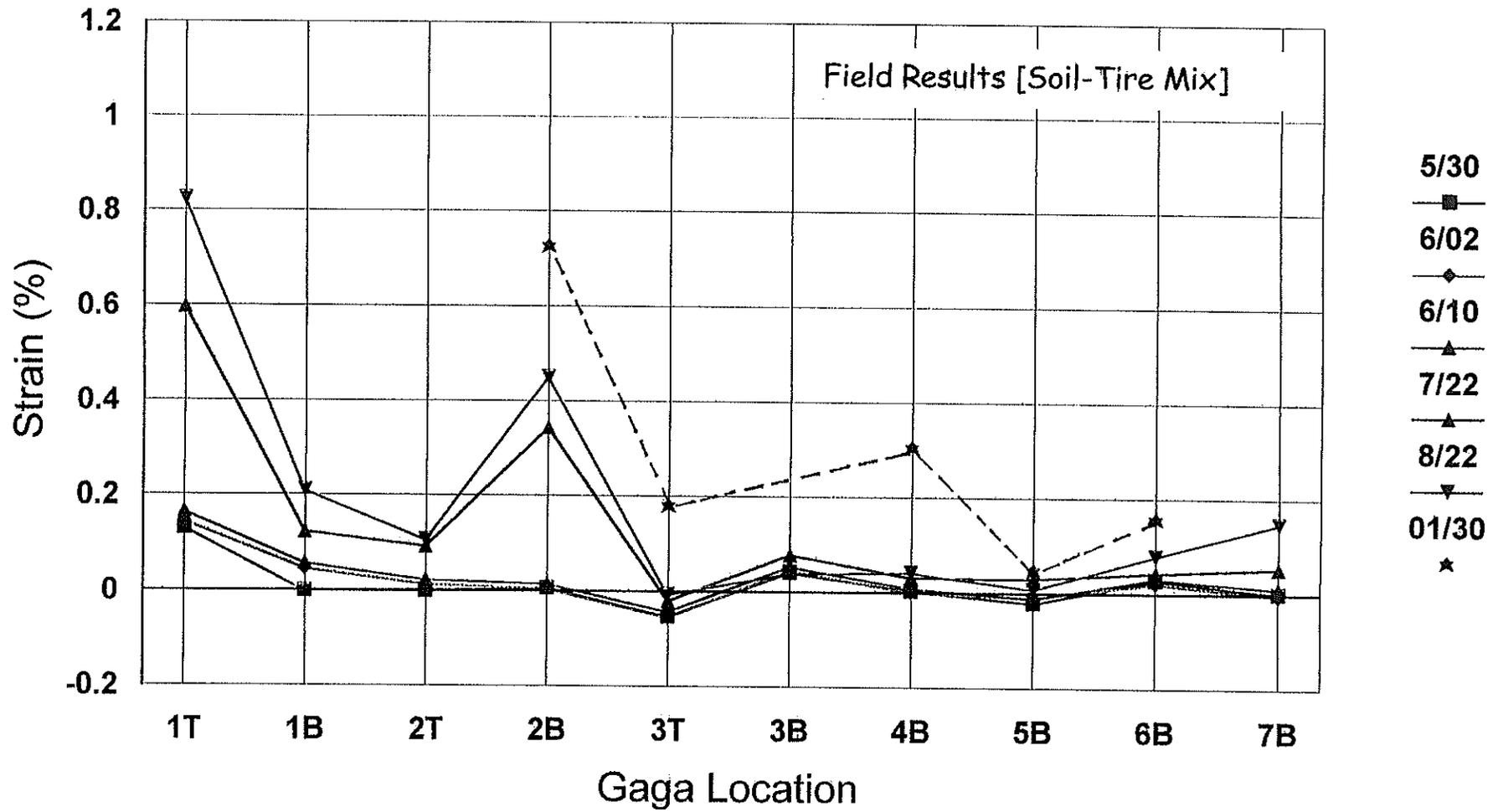
Figure B-5 Strain gage readings in soil-tire section
