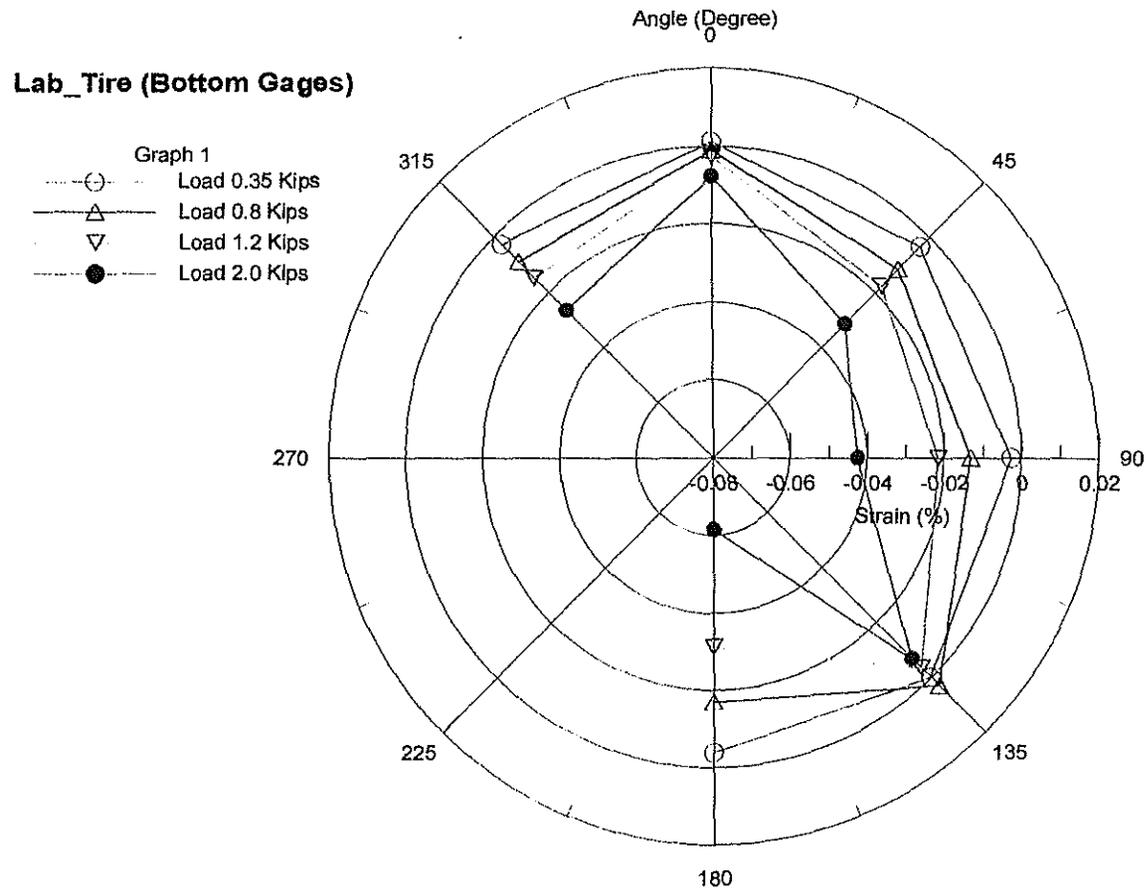
Figure 36. Strain measurements of bottom gages in tire fill
