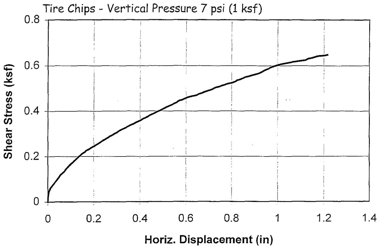
Figure A-3 Direct shear test on tire chips
