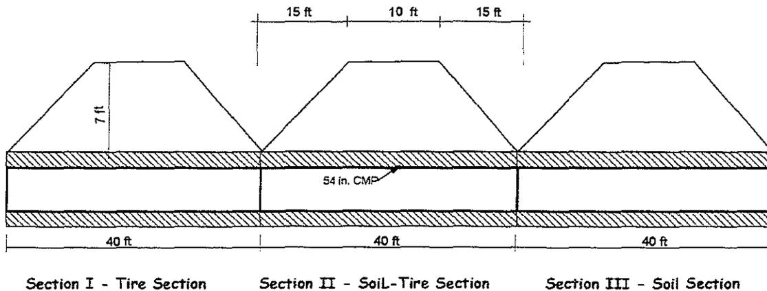
Figure 8. Longitudinal cross section of the test embankment
