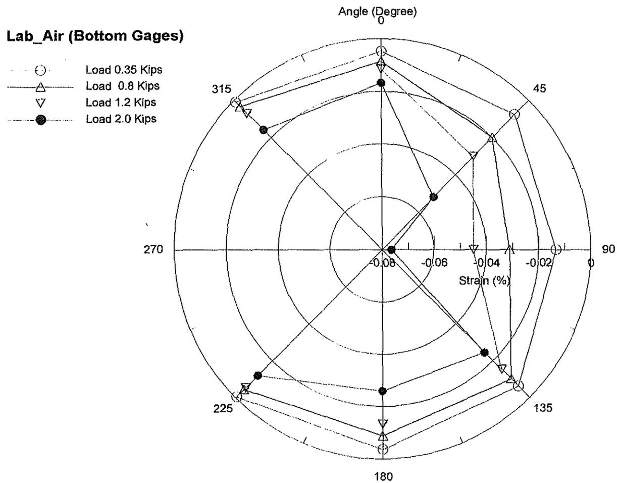
Figure 34. Strain measurements in bottom gages in in-air test
