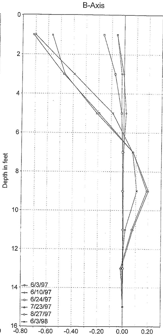
Figure B-2 Vertical inclinometer readings in soil-tire section
