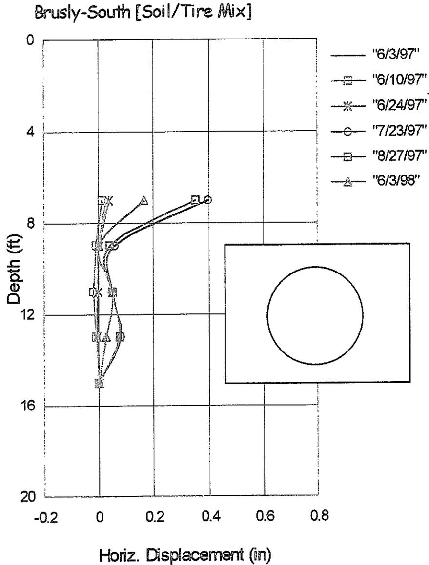
Figure 19. Horizontal soil displacement near the pipe in the soil-tire section
