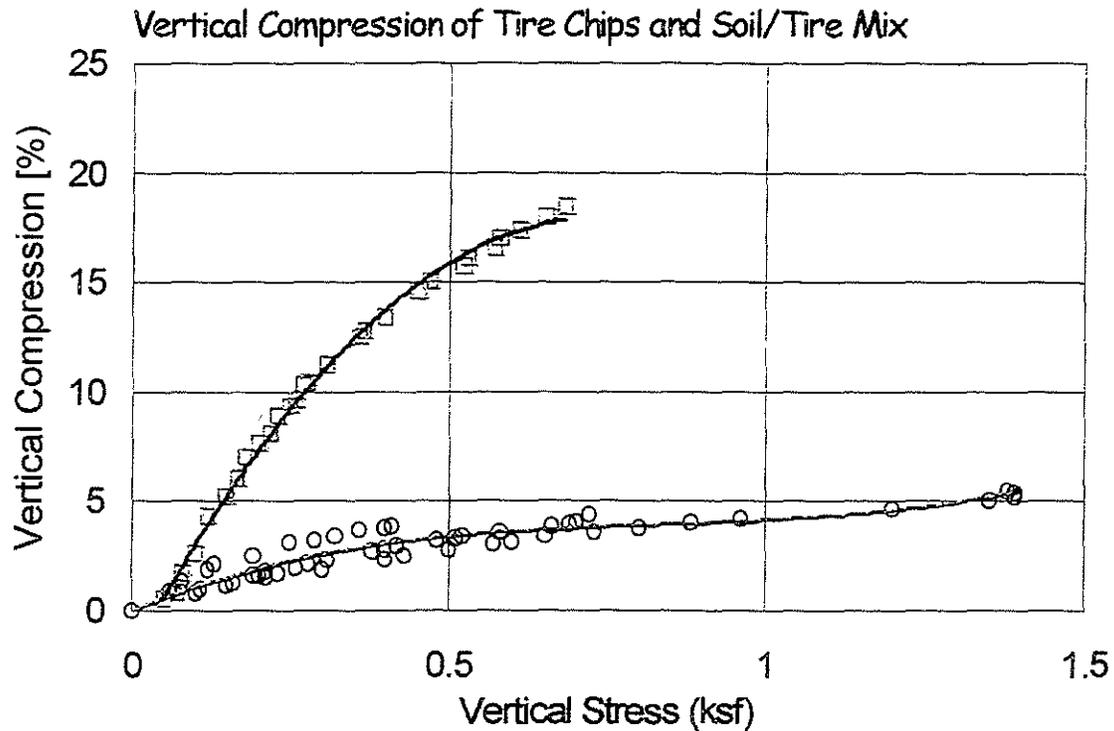
Figure 3. Compressibility of tire chips and soil-tire mix
