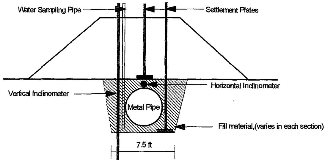
Figure 12. Layout of the field instrumentation
