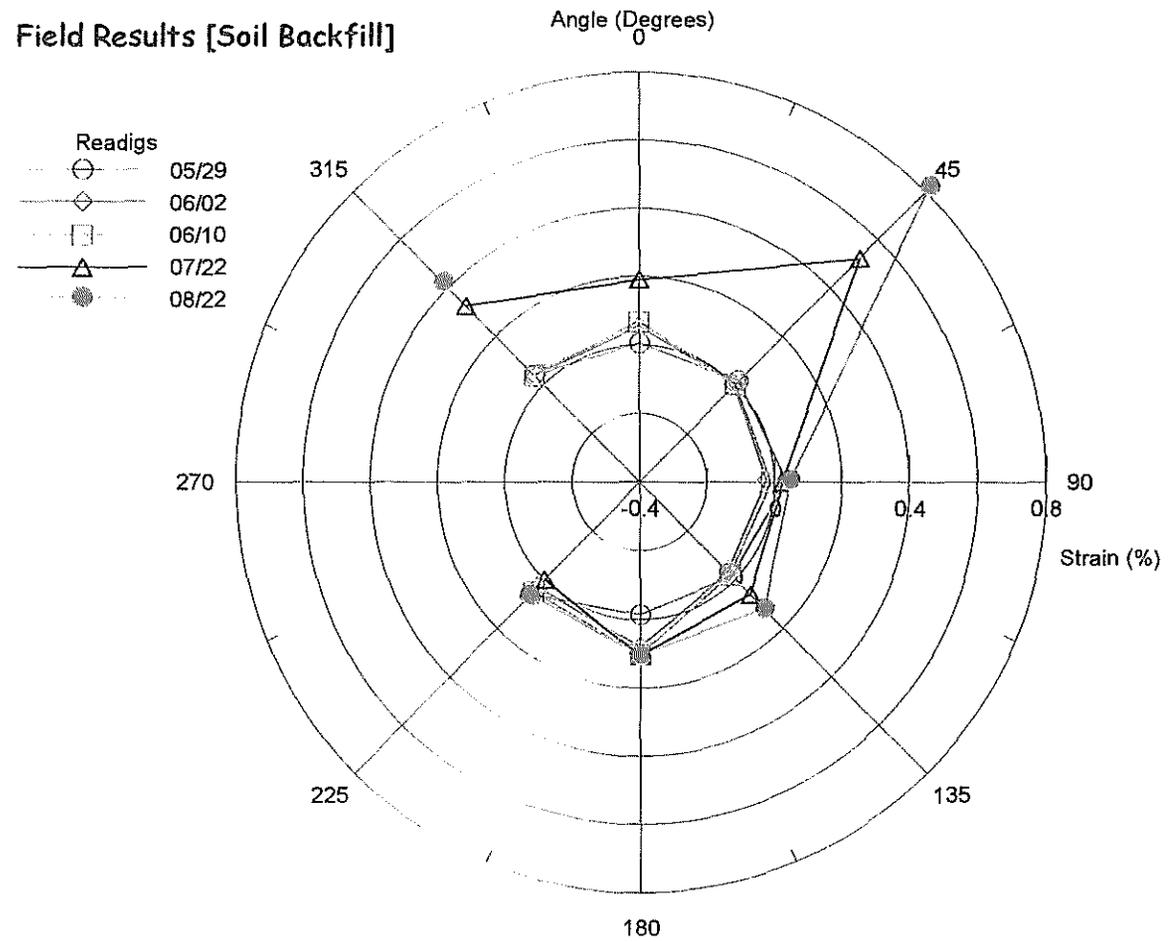
Figure 23. Strain measurements of bottom gages in the soil section
