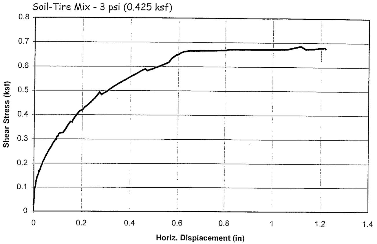
Figure A-4 Direct shear test on soil-tire mix
