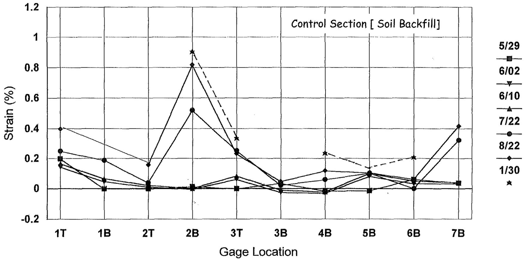
Figure B-6 Strain gage readings in soil section
