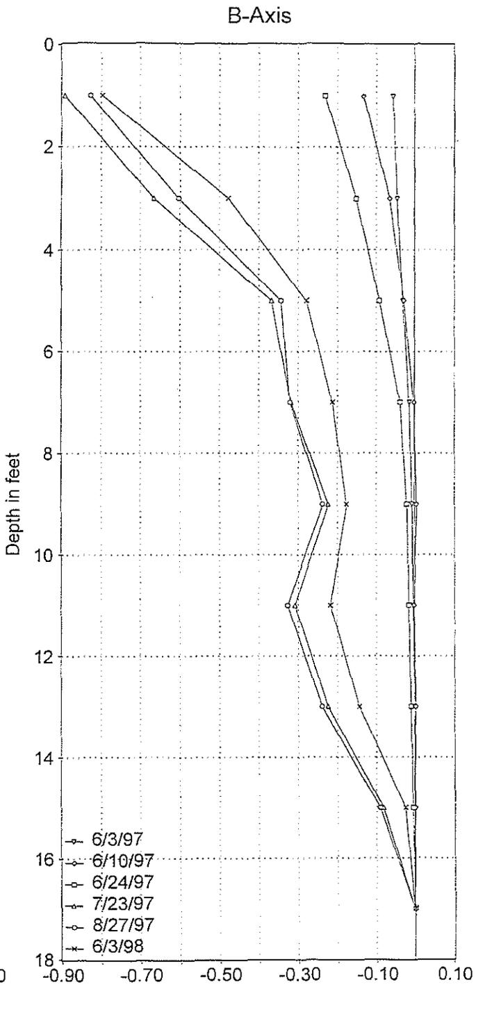
Figure B-1 Vertical inclinometer readings in tire-section
