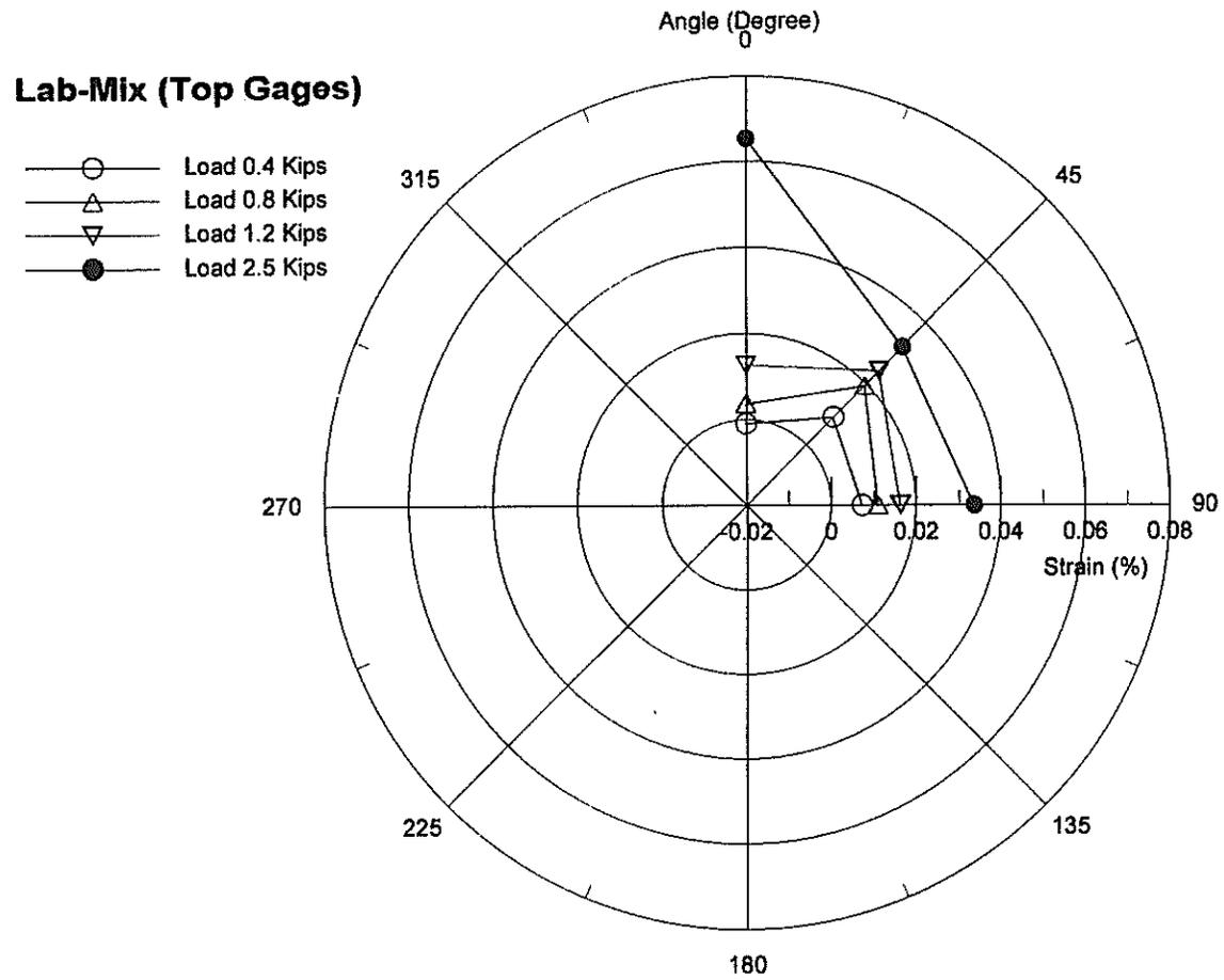
Figure 39. Strain measurements of top gages in soil-tire mix
