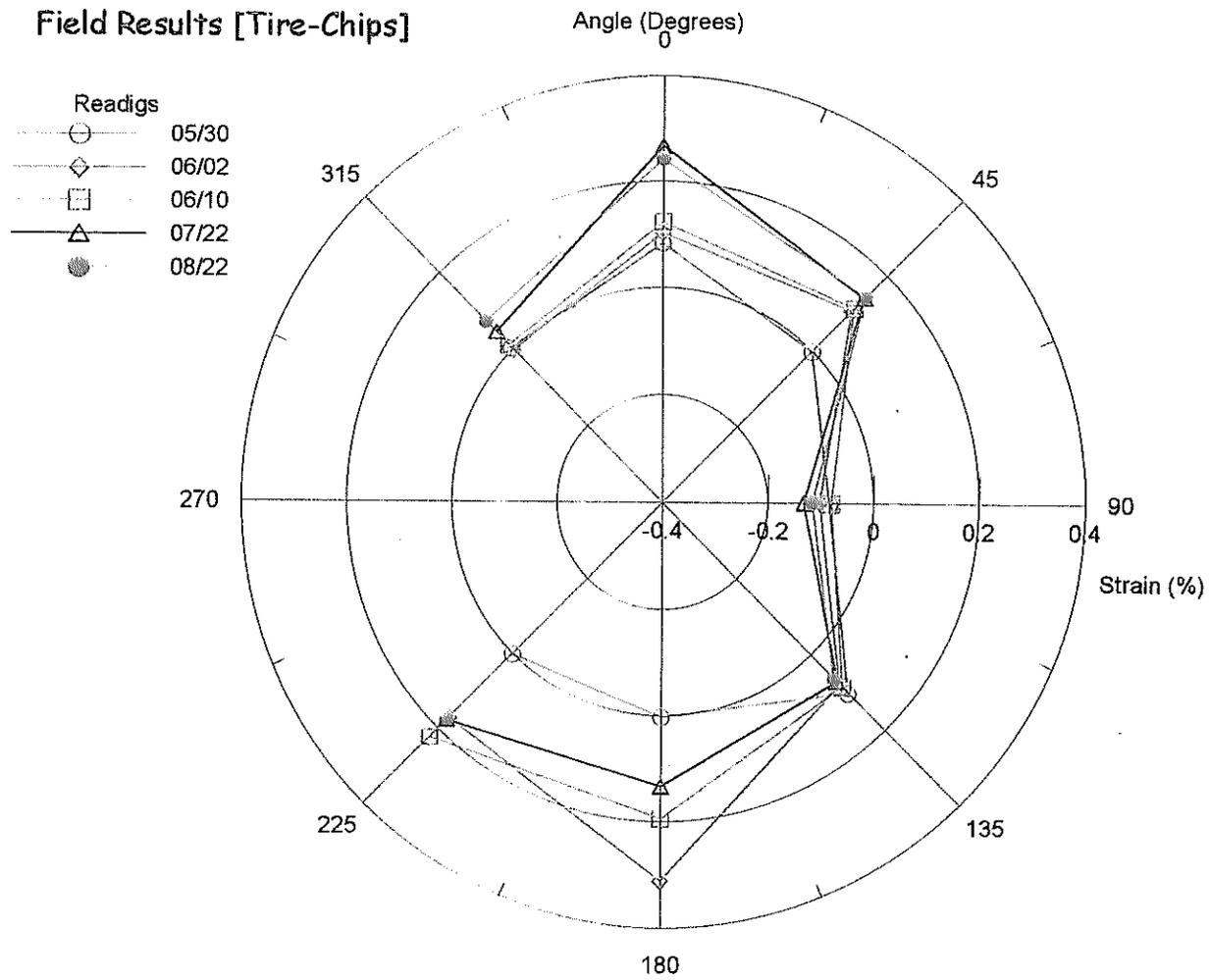
Figure 27. Strain measurements of bottom gages in the tire section
