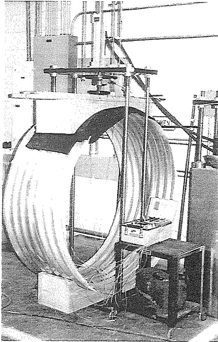
Figure 32. View of the in-air testing of the metal pipe
