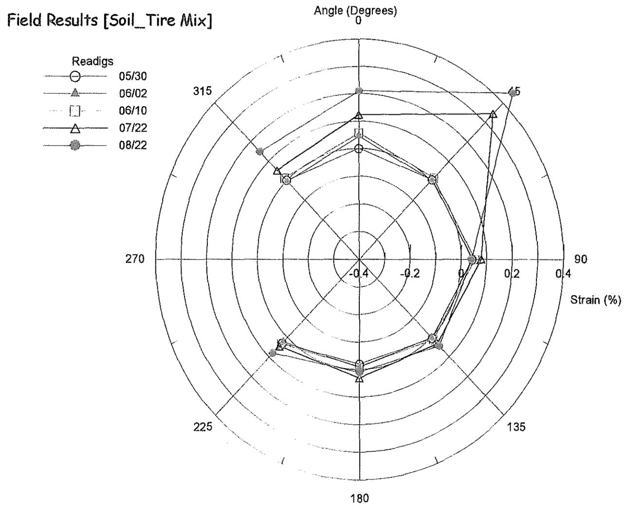
Figure 25. Strain distribution of bottom gages in the soil-tire section
