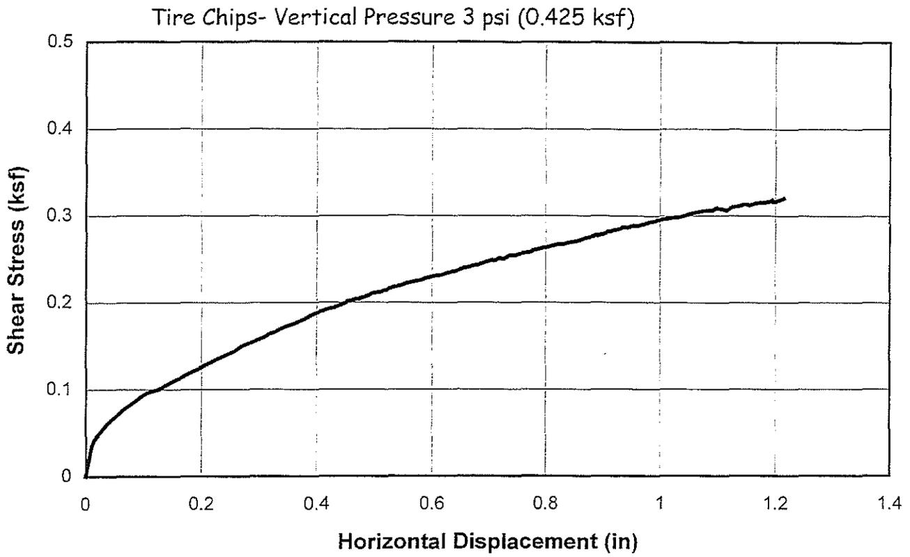
Figure A-1 Direct shear test on tire chips
