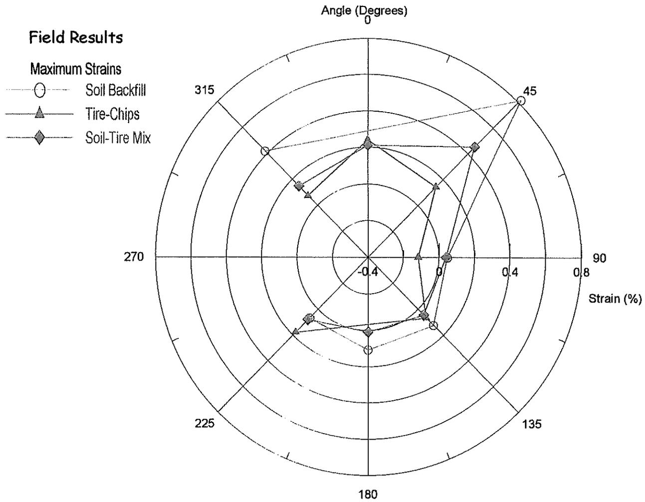
Figure 29. Comparison of strains in bottom gages in the three sections
