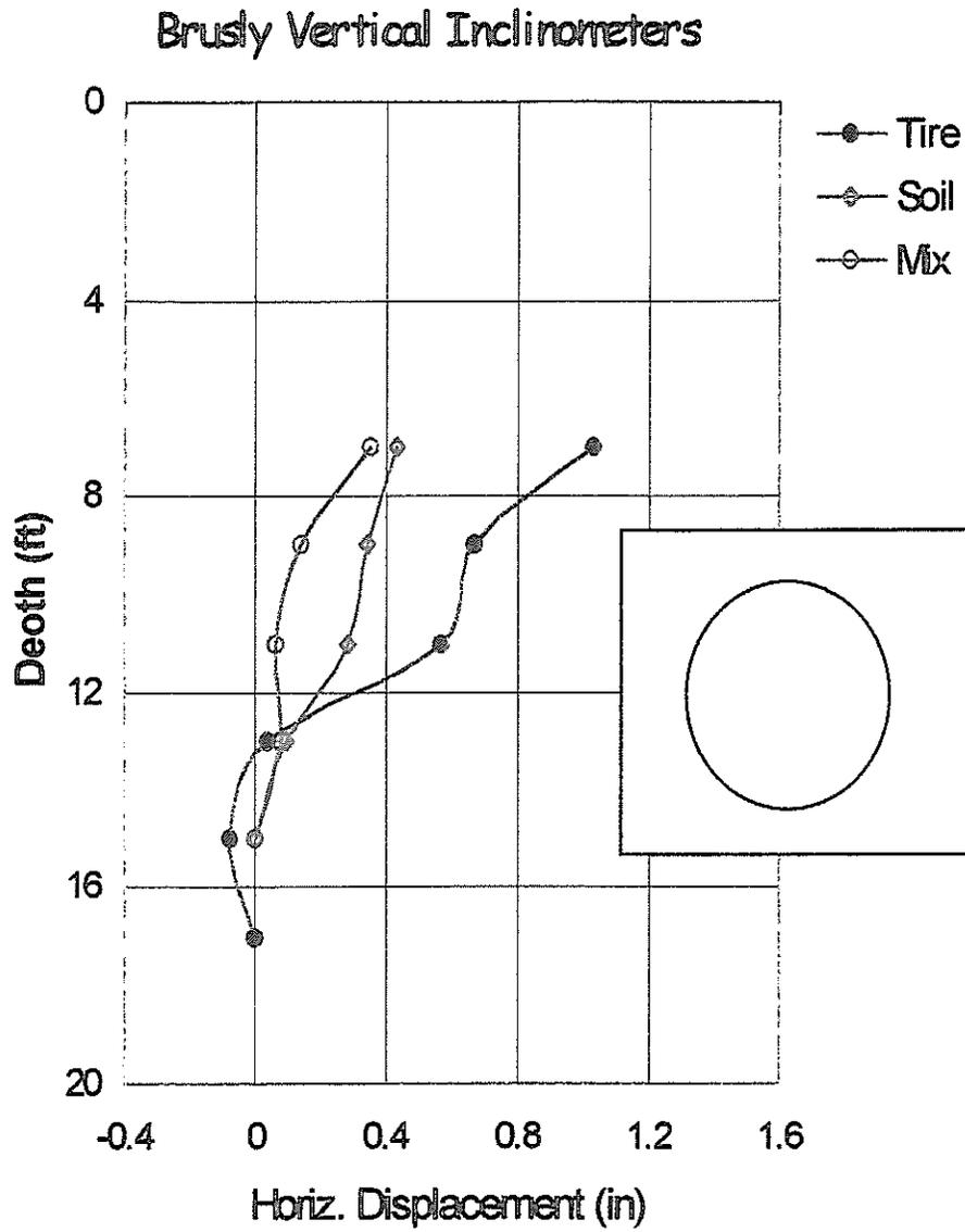
Figure 21. Comparison of horizontal soil movement in the three sections
