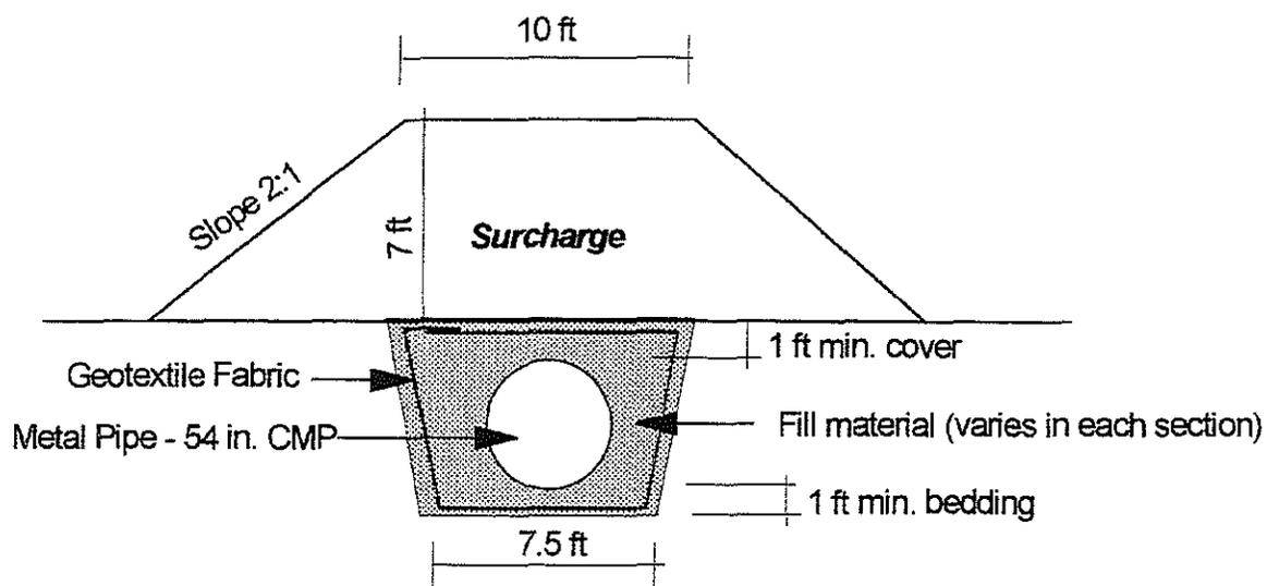
Figure 7. Typical cross section of the test embankment
