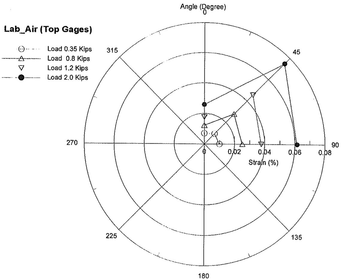
Figure 35. Strain measurements of top gages in in-air test
