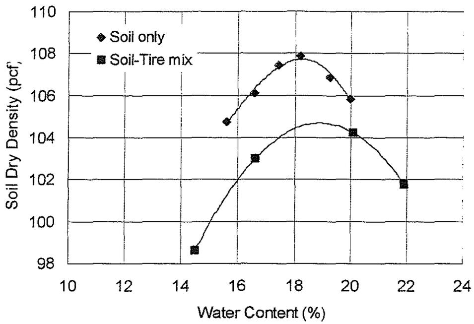
Figure 6. Moisture-Density relationship of the soil and the soil-tire mix
