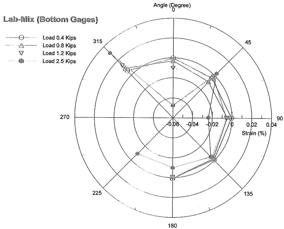
Figure 38. Strain measurements of bottom gages in soil-tire mix
