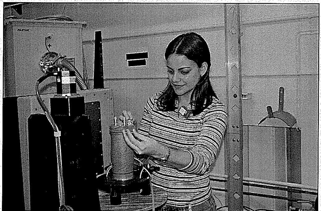
Preparing a sand specimen for computed tomography analysis
