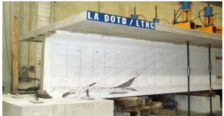
*Shear Test at CTL*
