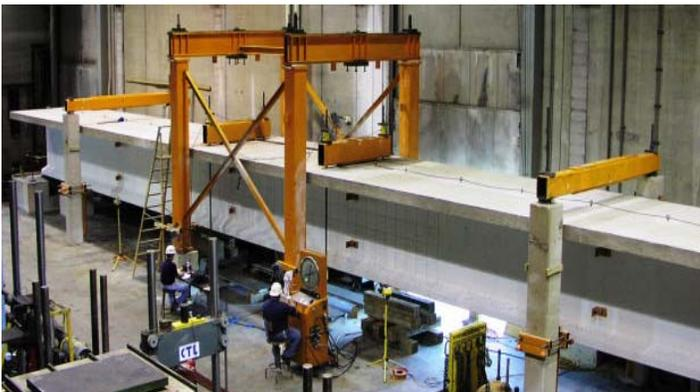
*Flexural Strength Test Setup*
