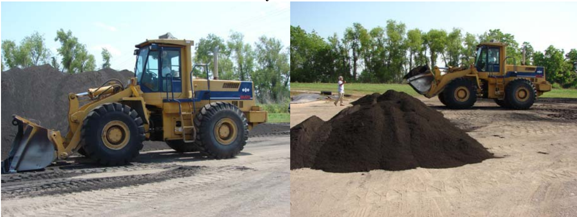
Figure 30 Komatsu WA420, front-end loader used to move stockpiled bottom ash
