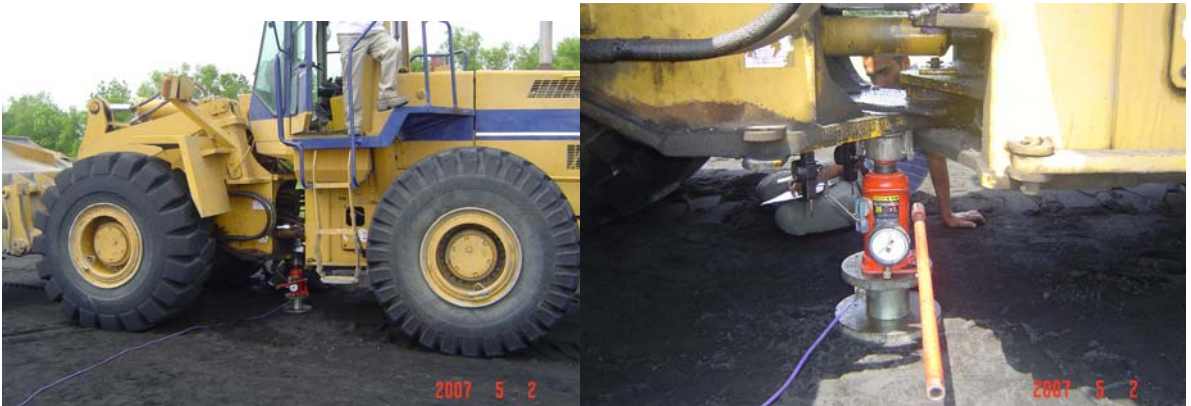
Figure 36 Plate load reaction vehicle and plate load setup
