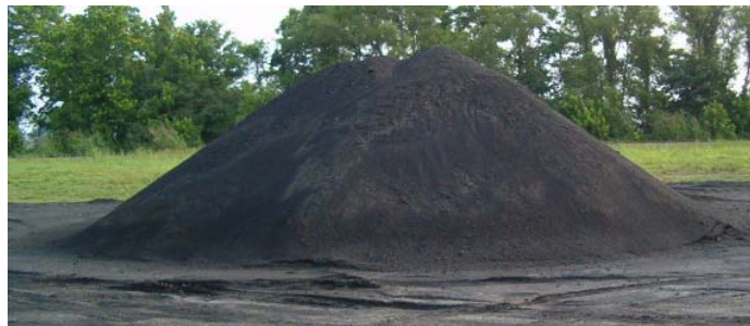
Figure 1 Stockpiled bottom ash for test section
