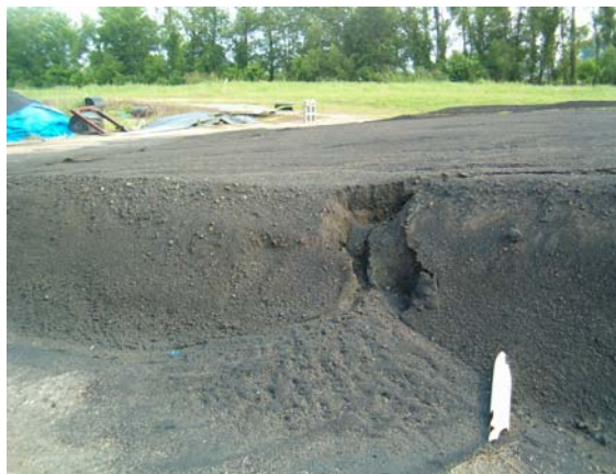
Figure 28 Erosion of test section
