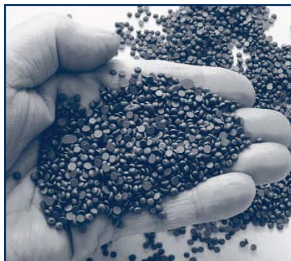
Shell Thiopave, a patented Shell additive containing sulphur, plasticizer, and other additives
