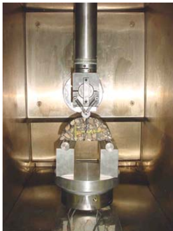
Figure 1 Semi circular bend test setup
