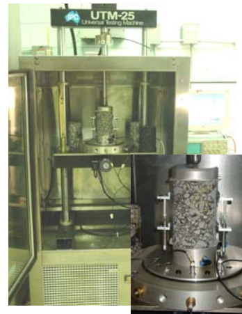
Figure 2 Dynamic modulus test set up
