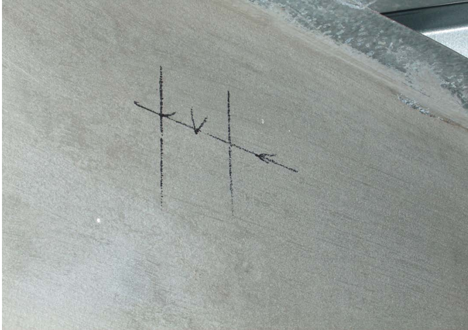
Figure 187 Initial marking on the continuity diaphragm for placing transducer
