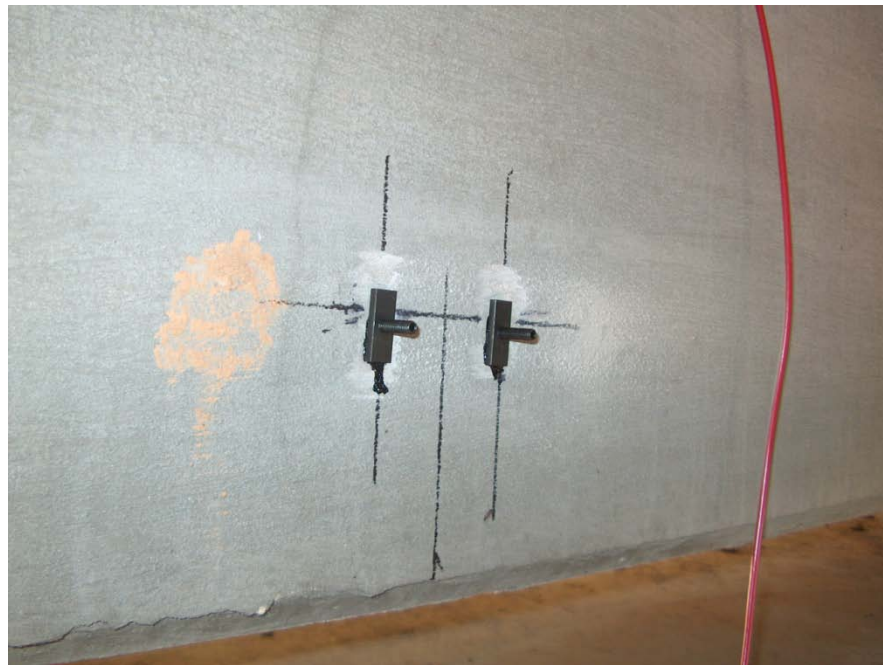
Figure 194 Tabs on the continuity diaphragm after removing the transducer
