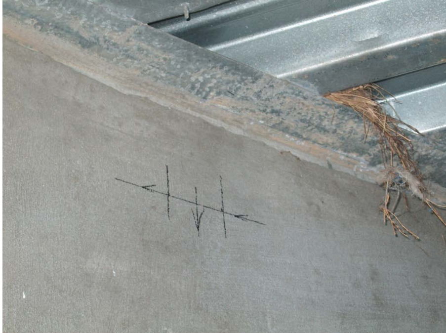
Figure 195 Initial marking on the continuity diaphragm for placing transducer
