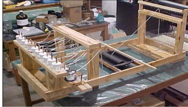
Figure 2 FRP grid manufacturing system setup
