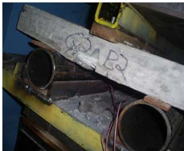
Figure 21 Manually-fabricated FRP grid reinforced slab failure mode
