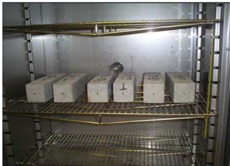
Figure 15 Specimens placed inside the oven set at 200^{\circ}\text{F}
