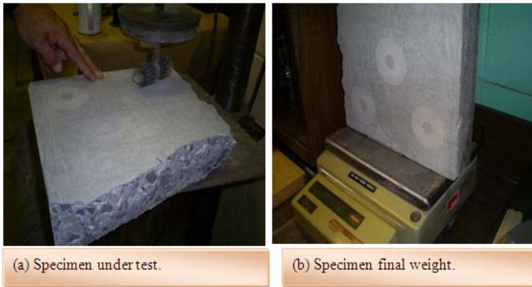
Figure 13 Surface abrasion test setup
