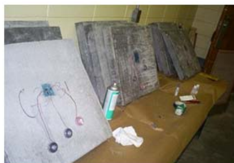
Figure 8 Strain gages pasted on the slabs
