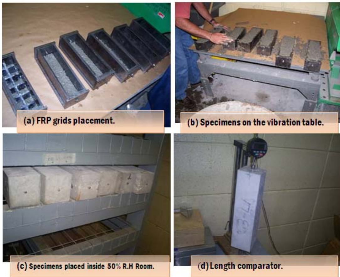
Figure 14 Shrinkage test procedures
