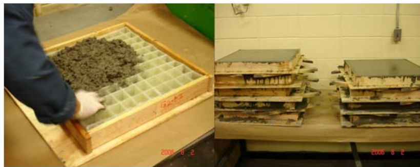
Figure 7 Pouring concrete into a lab-made FRP grid reinforced concrete
