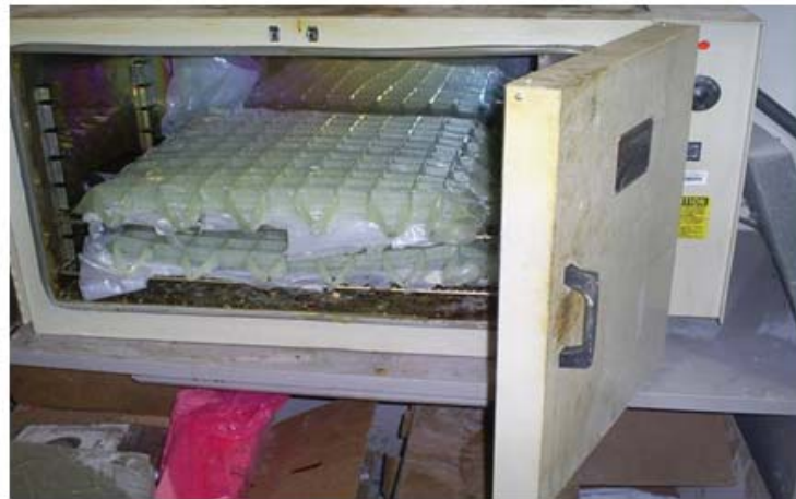
Figure 6 The fabricated FRP grids curing inside the oven
