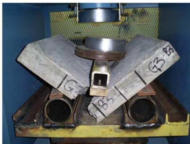
Figure 17 Plain concrete failure mode
