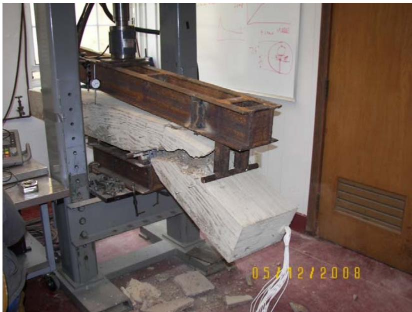
Figure 56 Beam 1 at collapse
