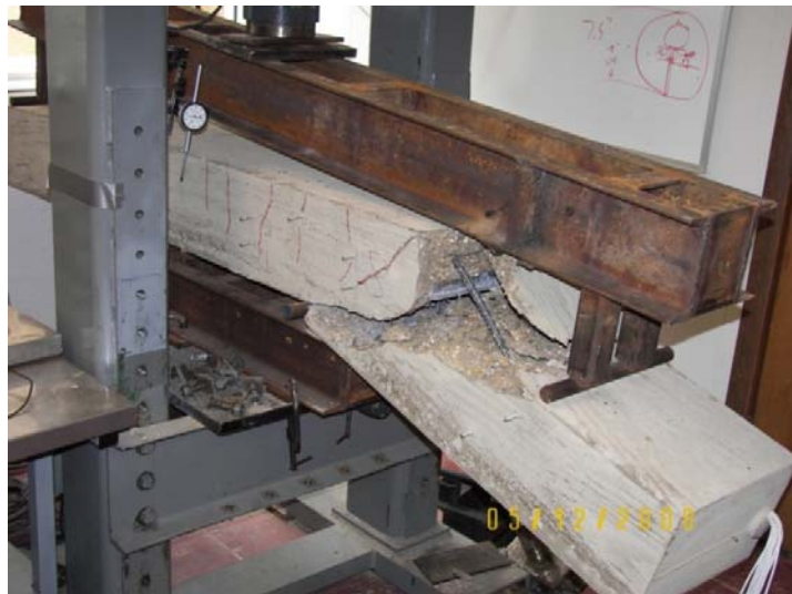
Figure 57 Beam 2 at collapse
