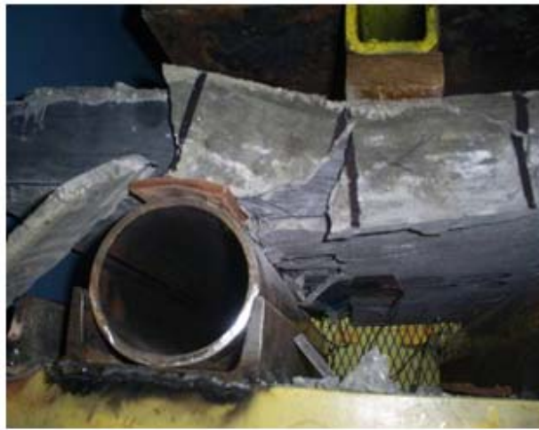
Figure 19 Commercial FRP grid reinforced slab failure mode
