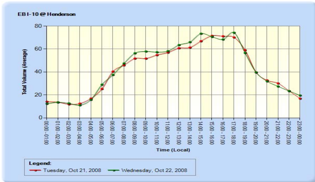
Figure 10 Hourly volumes for two days from detectors on EB I-10 at Henderson
