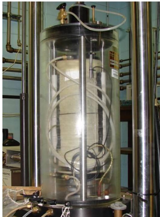
Figure 3 Setup of a permanent deformation (P-D) test
