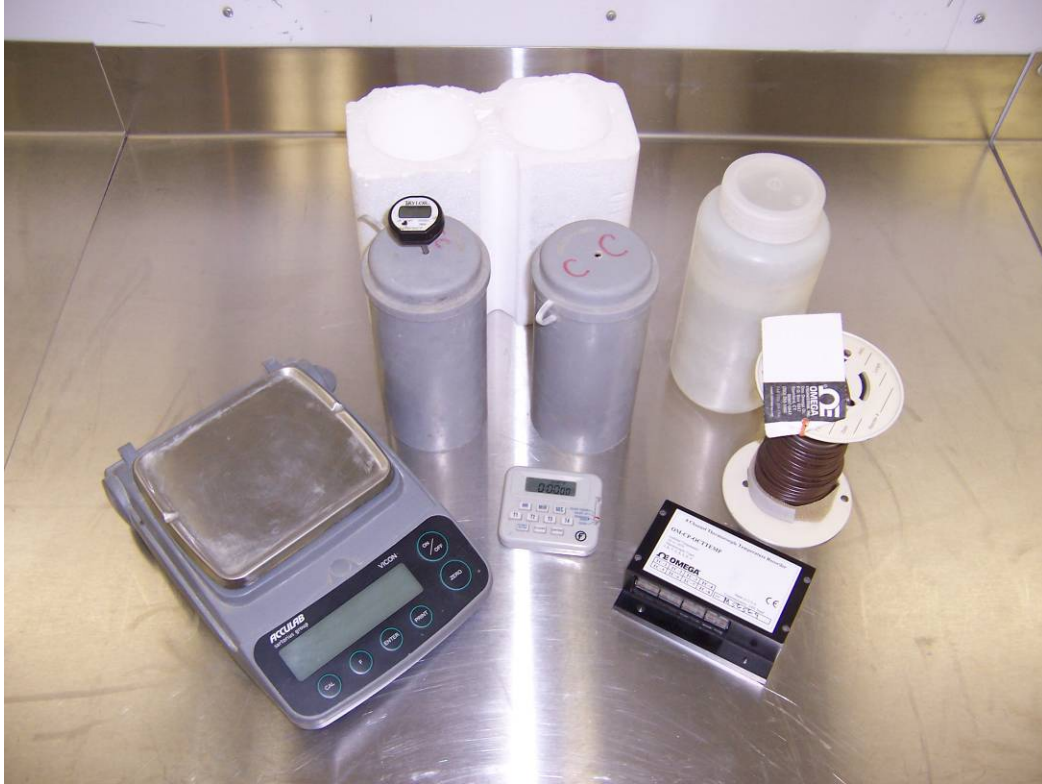
Figure 5 Laboratory test equipment used to conduct the quick heat generation test
