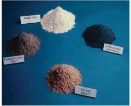
Another benefit of replacing Portland cement with fly ash and slag is a reduced carbon footprint during production of the cementitious material. Production for each ton of Portland cement for concrete pavement emits 0.92 tons of carbon dioxide. As byproducts of other industries, emissions due to production of fly ash and slag are negligible from the viewpoint of concrete pavement construction.
