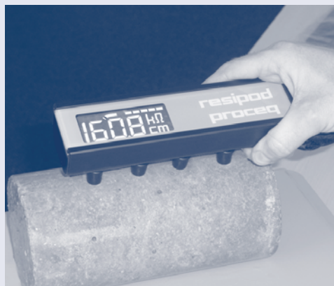
Surface resistivity meter
