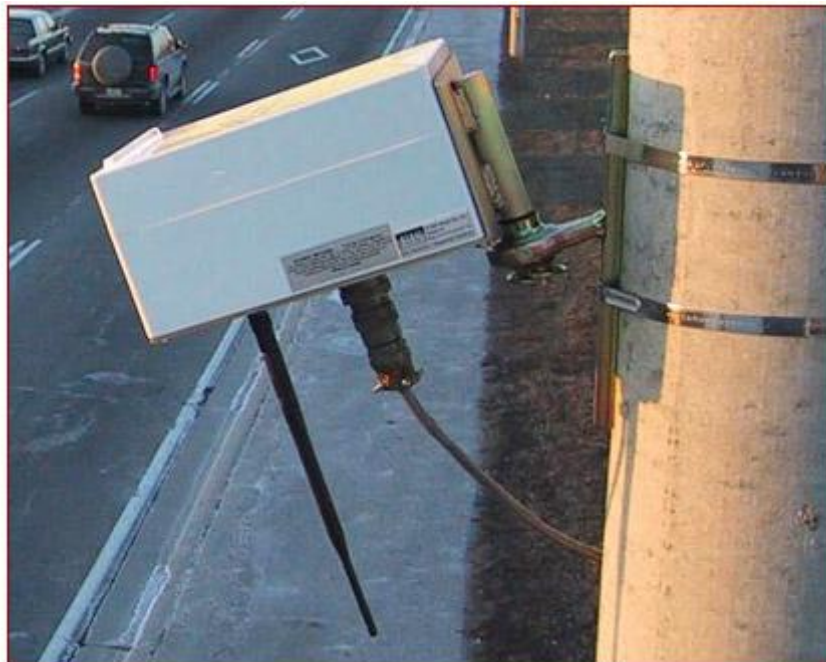
Figure 5 A snapshot of a roadside mounted RTMS device
