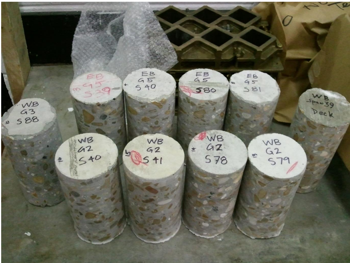
Figure 1 Girder cores from the US 90 Bayou Ramos Bridge
