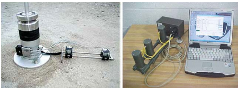
Figure 1 Left—Light weight deflectometer, right—Portable seismic pavement analyzer
