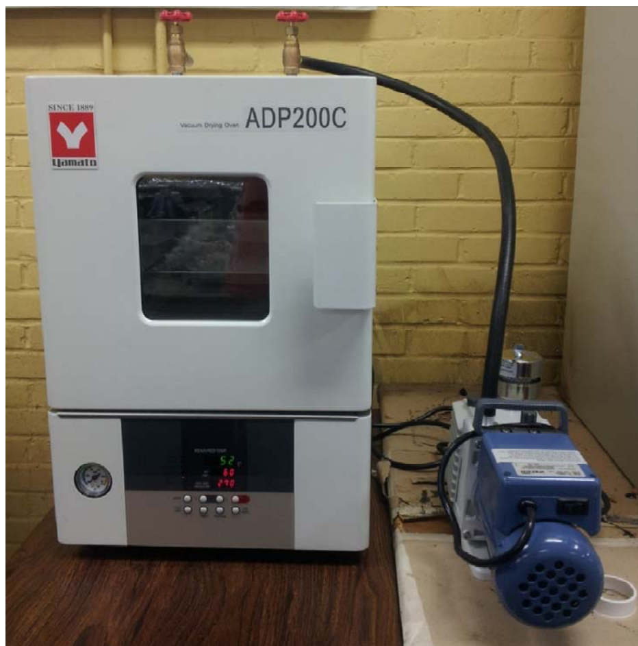
Figure 3 Setup for vacuum drying method (vacuum drying oven with pump)
