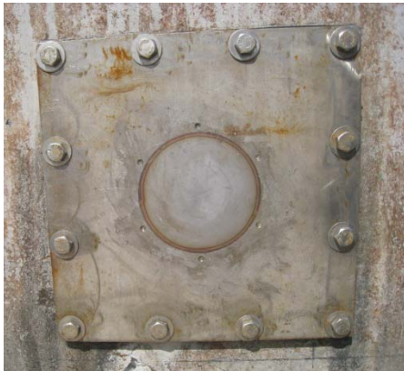
(c) Water pressure cell
