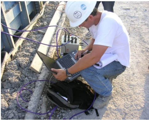
(c) Monitoring Strain Gauges
