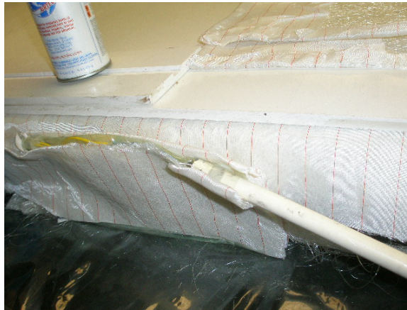
Figure 112 Fiber cables in packaging secured to the panel edge with ply peel fabric
