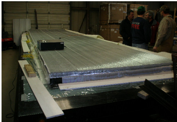
Figure 108 Deck covered with longitudinal pieces of hardwire
