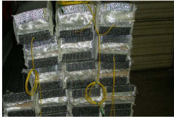
Figure 105 Wrapping of balsa wood beam with E-glass
