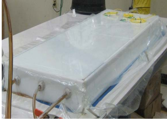
Figure 113 Vacuum infusion process
