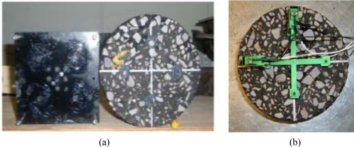
Figure D. 4 Instrumentation: a) installation of gage point b) mounted extensometer
