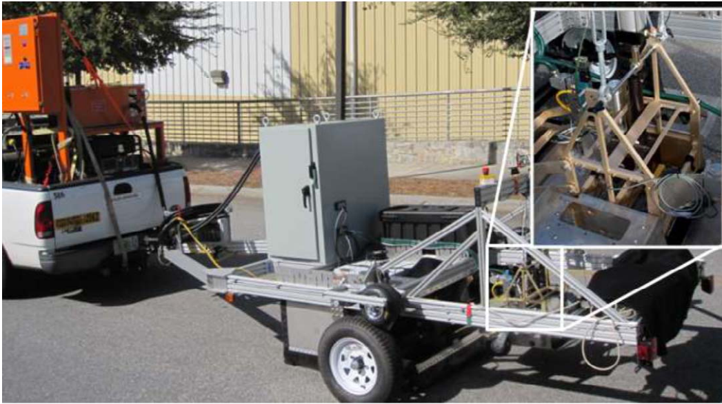
Figure 11-1 Prototype Crack Sealing Hardware Developed by GTRI and GDOT (Holmes, Holcombe, Daley, Coli, & Robertson, 2010)
