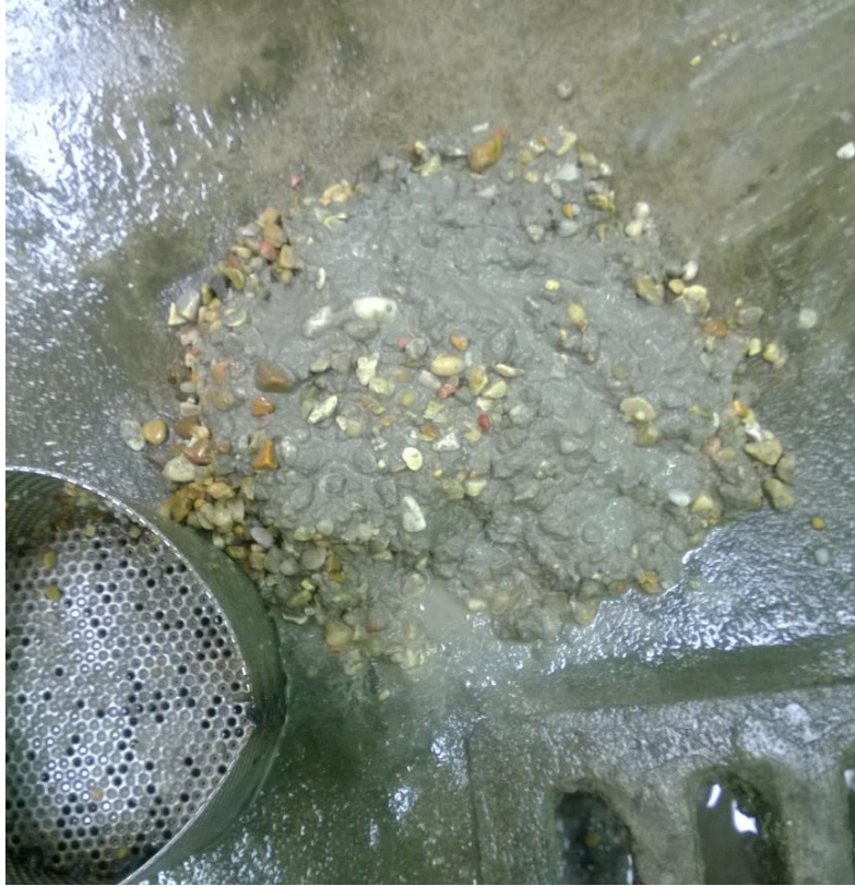
Figure 7 Washout test result for a No. 8 pea gravel mixture incorporating a VMA showing cement paste
