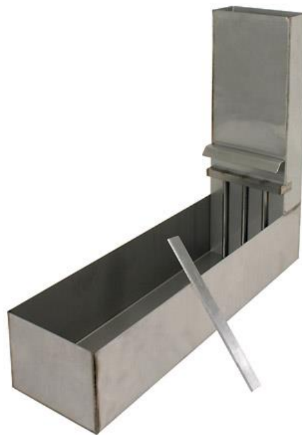
Figure 1 L-box test apparatus
