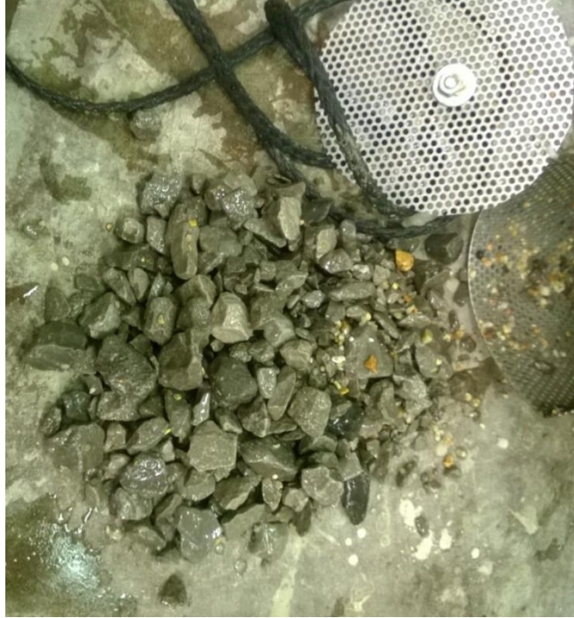
Figure 5 Washout test result for a No. 67 stone mixture showing no cement paste
