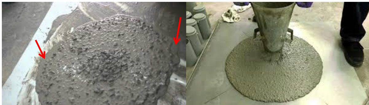
Figure 2 Left: Segregated SCC with a mortar halo indicated by red arrows; Right: Proper SCC consistency
