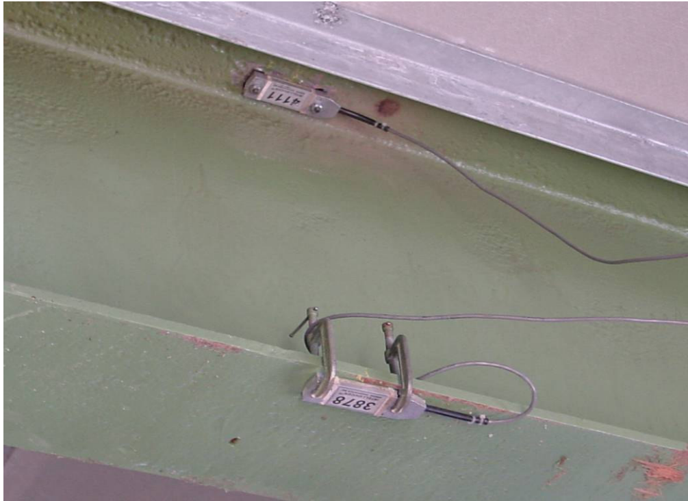
Figure 60 Strain Transducers Mounted on Steel Girder
