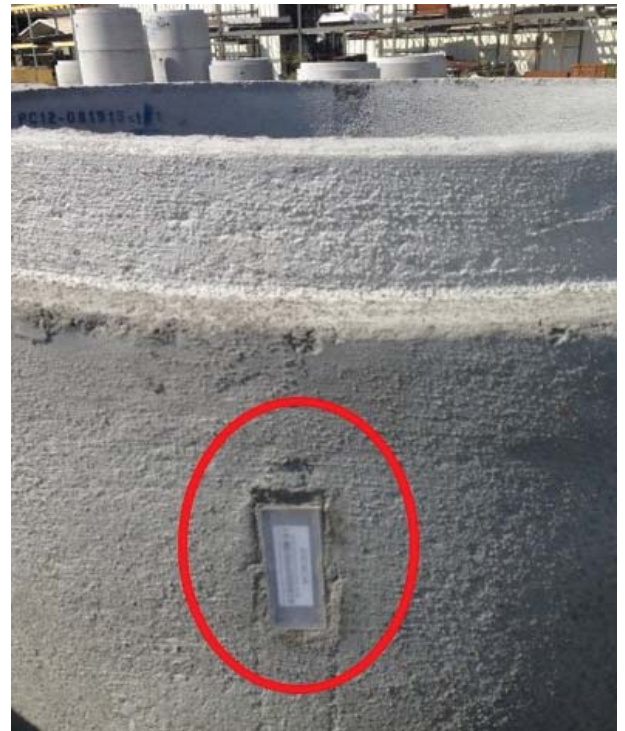
RFID tag in concrete pipe
