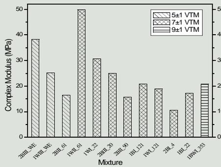
Complex shear modulus of frequency sweep at constant height test at 0.01 Hz and 48°C
