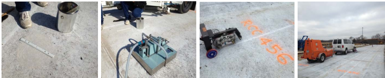
(a) Sand Patch Test (b) Dynamic Friction Tester (c) Walking Profiler (d) FWD Testing
