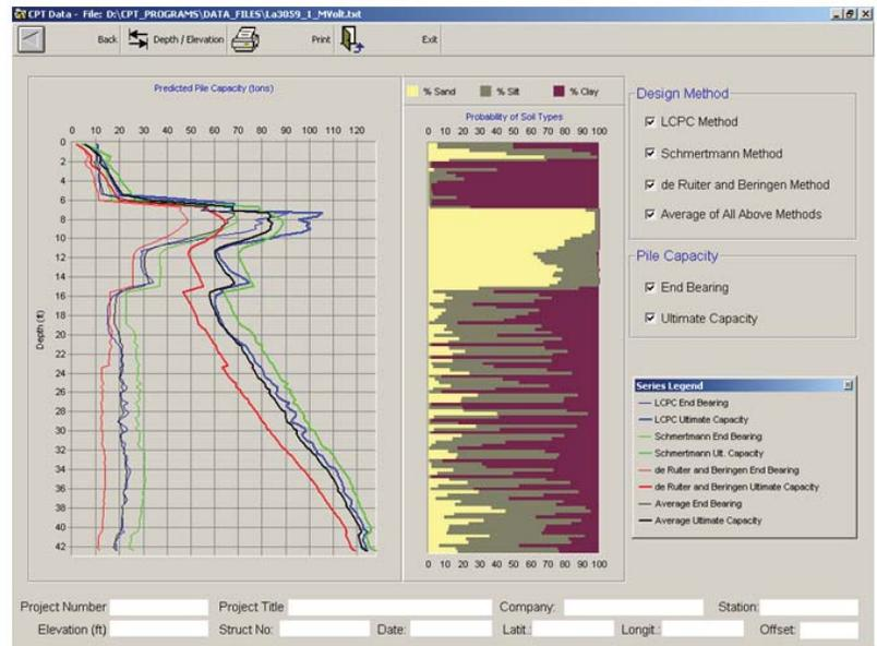
compare pile resistance measured with load tests and pile resistance predicted with CPT data; and perform statistical analyses to evaluate and rank the different CPT pile design methods.
