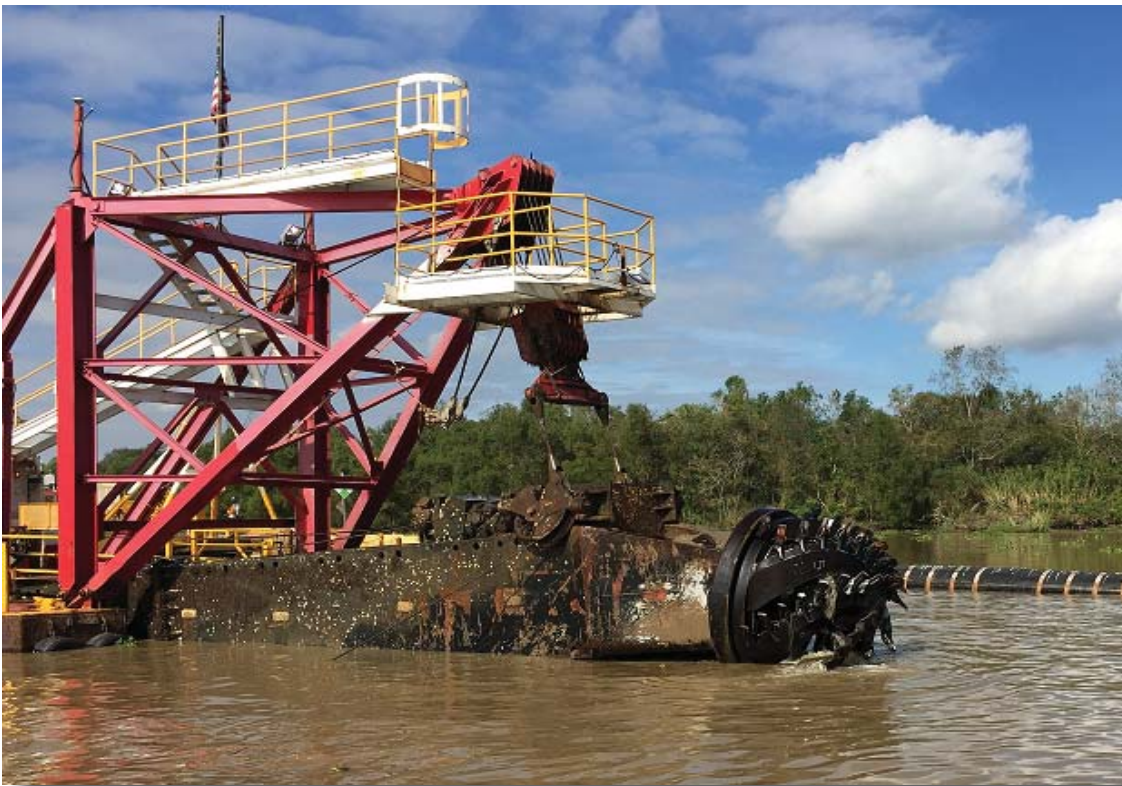
Figure 1 A dredge near Morgan City in November 2015 with the cutter head exposed
