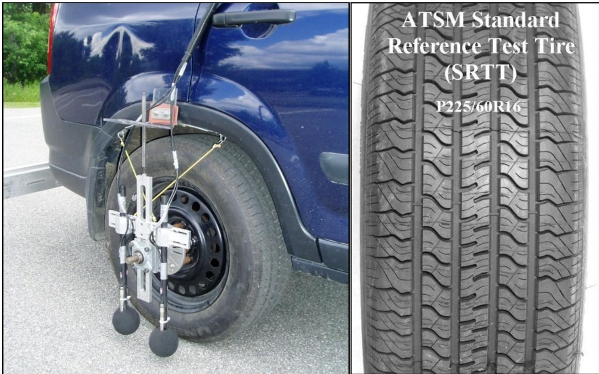
Figure 10. Photo. OBSI dual-probe system and the SRTT.
