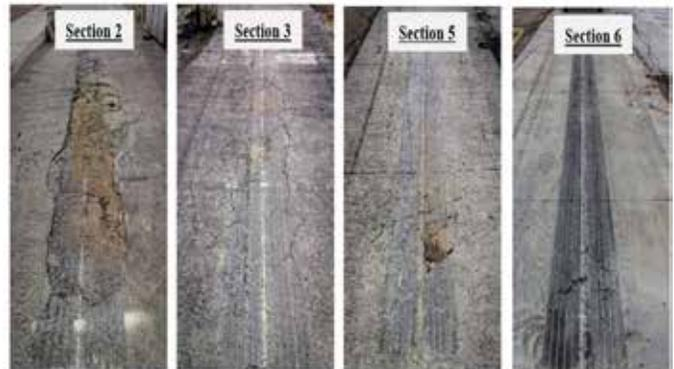
CRACKING FAILURE THAT OCCURRED DURING TESTING
