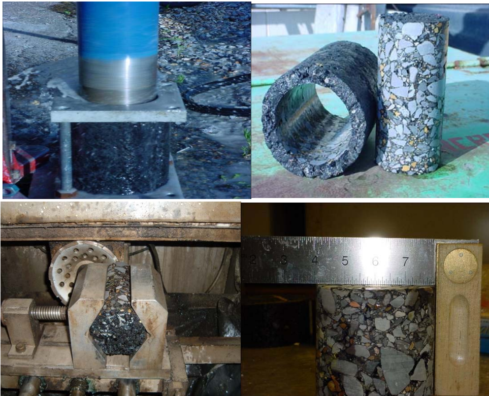
Figure 5 Specimen preparation for the dynamic modulus test
