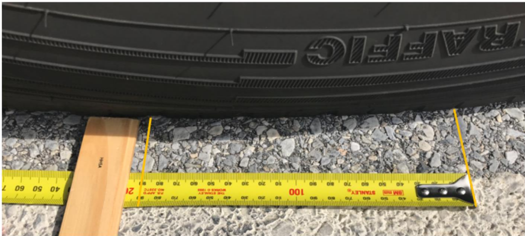
(b)TSD tire dimensions in longitudinal (traffic) direction
