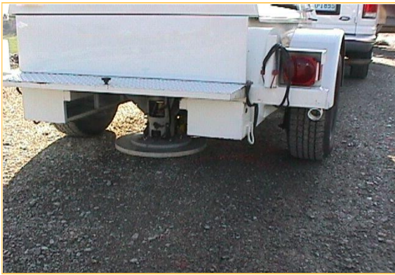
(a) FWD testing using a circular plate
