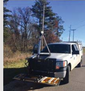
Figure 1 (left): FDH rapid bridge deck scanning
