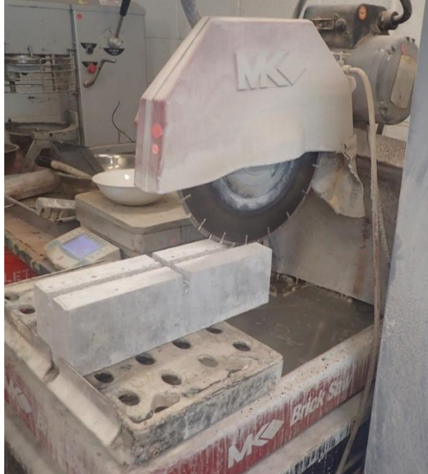
Figure 40. Saw-cutting of longitudinal groove.
