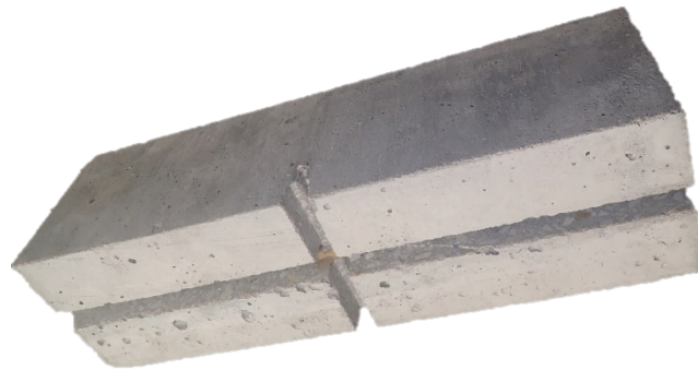
Figure 41. Axonometric view (from the bottom) of a bond characterization specimen with 1-in notch and longitudinal groove.
