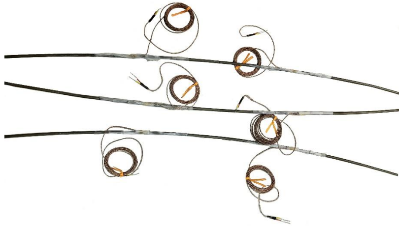
Figure 42. NiTiNb wires prepared for placement in the grooves: Type K thermocouples' probes were affixed to the wire surface followed by wrapping with scotch tape to provide debonded length.
