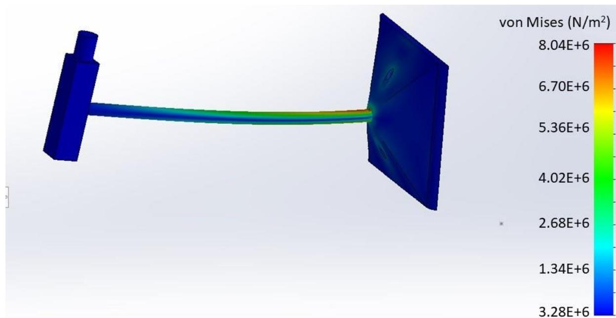
**Figure 3.** Finite element stress analysis of a single motor-arm-sidewall assembly in order to determine maximum stress magnitude and location.
