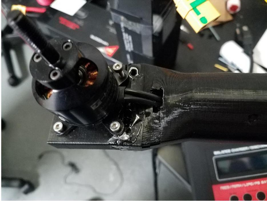
**Figure 8.** Close-up of the broken motor mount after a repair attempt was made. Fracture was across the two bolts holes on the right.
