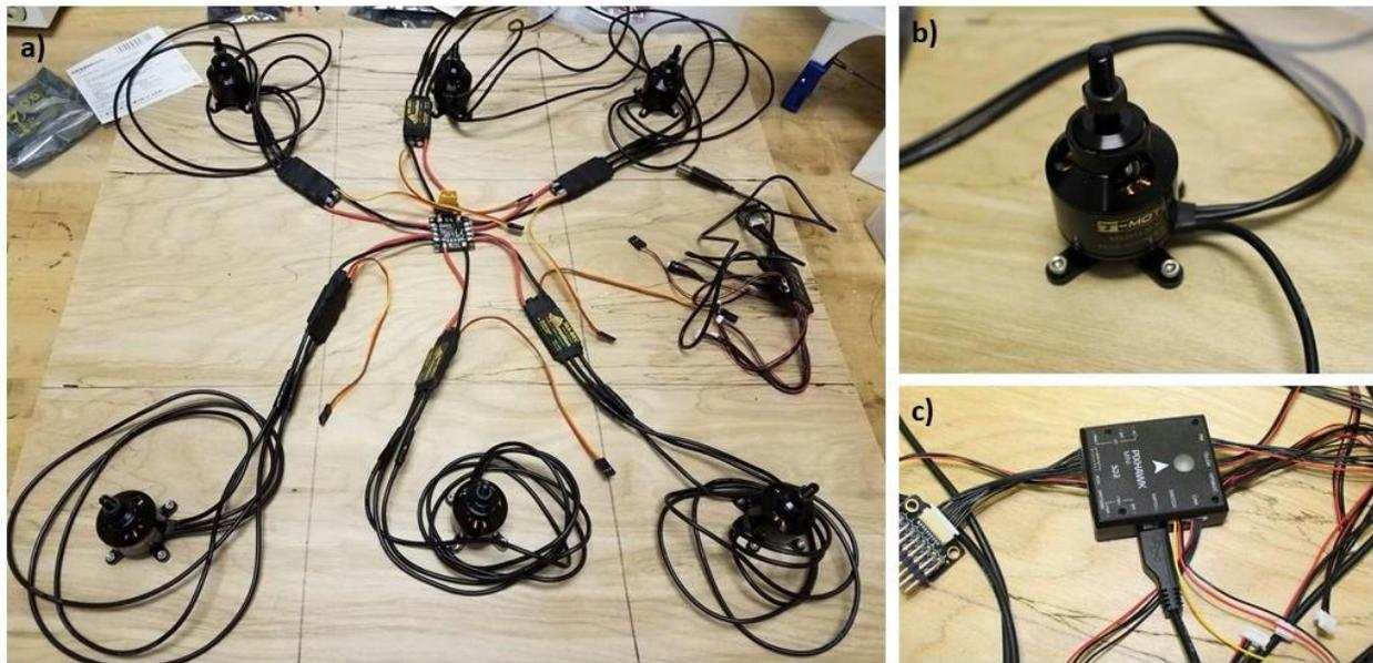
**Figure 5.** UAV electrical component wiring and integration activities. a) The six motors mounted to a benchtop integration setup along with electronic speed controllers and a power distribution board. b) A closeup of one of the six motors. c) The 3DR Pixhawk Mini flight controller, ready for programming via the USB uplink cable and associated laptop (not shown).
