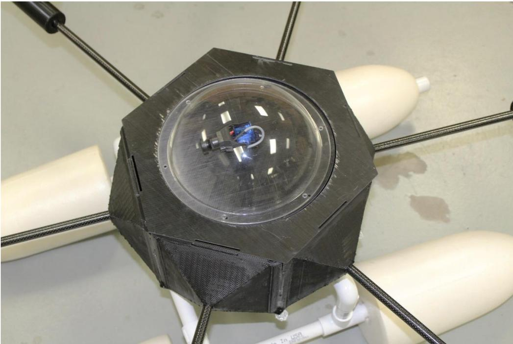
**Figure 7.** Close-up of the fully assembled UAV prototype hexcopter.
