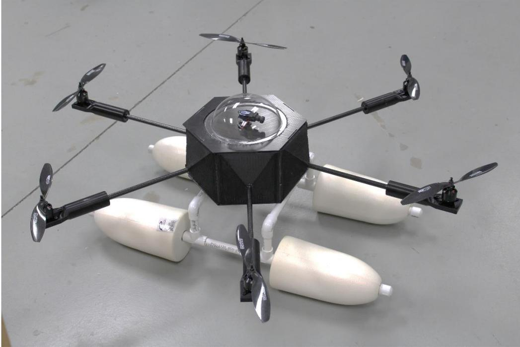
**Figure 6.** The fully assembled UAV prototype hexcopter.
