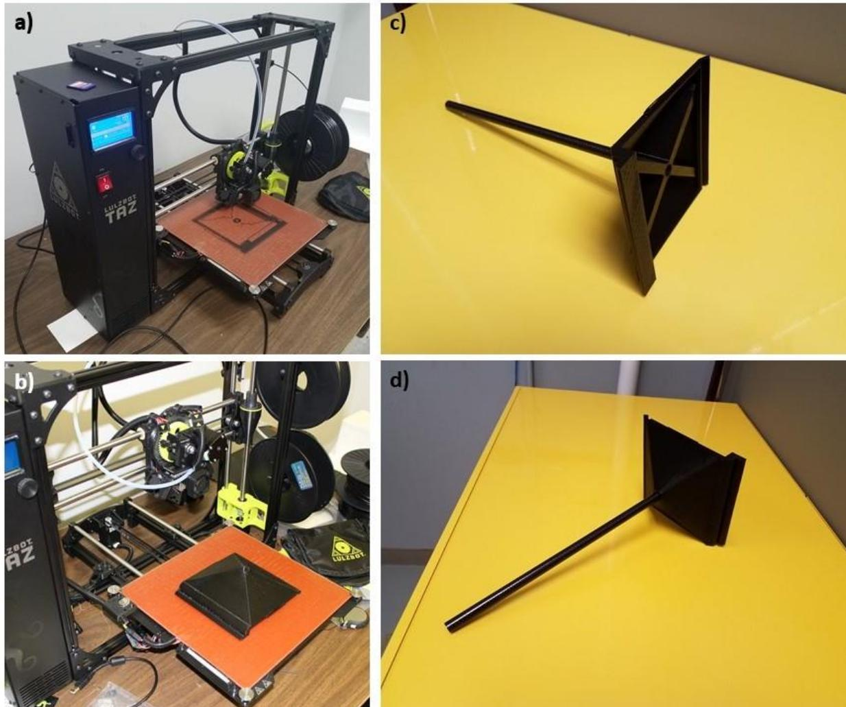
**Figure 4.** UAV body fabrication activities. a) A 3D print of one sidewall beginning. b) The completed sidewall. c) Inside view of the sidewall with graphite tube “arm” inserted. d) Outside view of the same sidewall/arm assembly.
