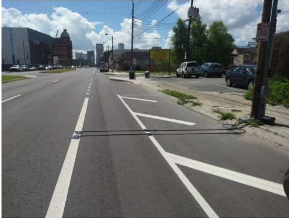
Figure 1 Tulane Avenue count equipment configuration, inbound
